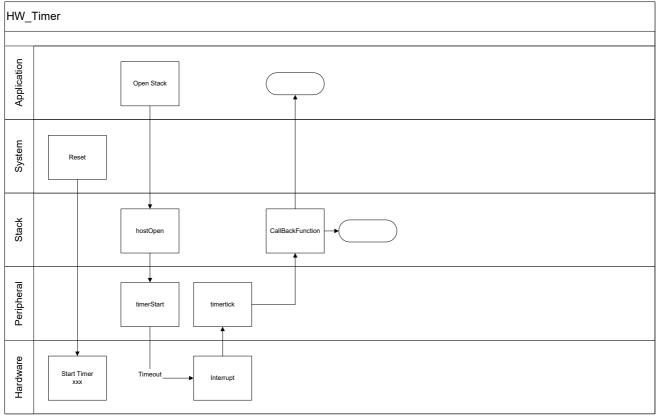
Figure 4-13 Base Hardware Timer Operation
