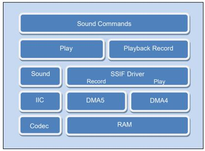
Figure 4-42 Sound Function Hierarchical Software Layer
