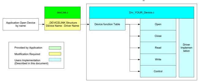
Figure 3-6 Device Linkage
