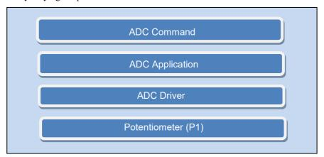
Figure 4-1 ADC Hierarchical Software Layer
