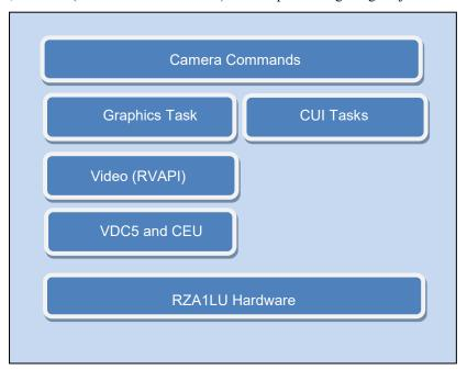
Figure 4-34 Camera Hierarchical Software Layer
