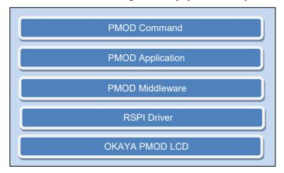
Figure 4-5 PMOD Hierarchical Software Layer
