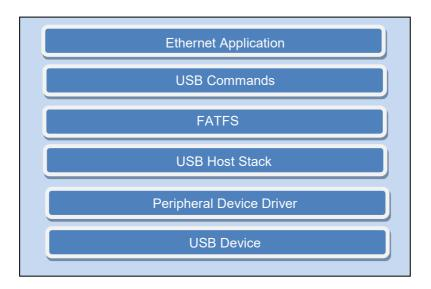
Figure 4-7 USB Hierarchical Software Layer
