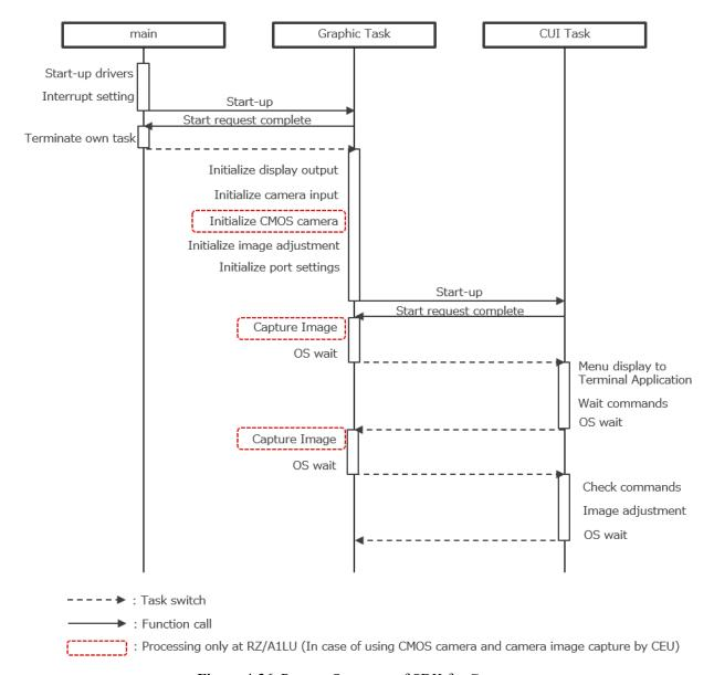
Figure 4-36 Process Sequence of SDK for Camera
