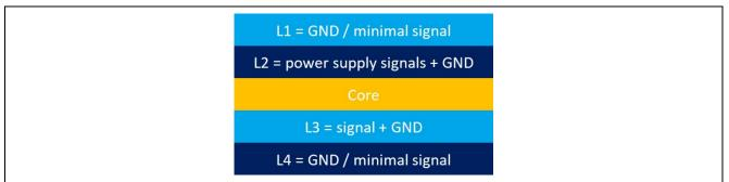
Figure 12. 4-Layer PCB Example
