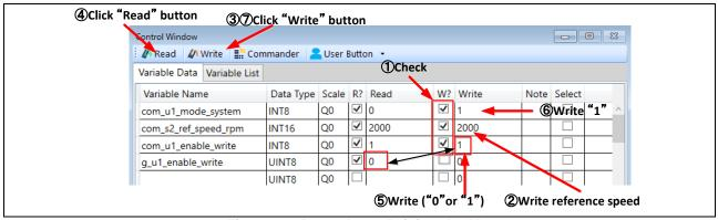
Figure 4-2 Procedure - Driving the Motor
