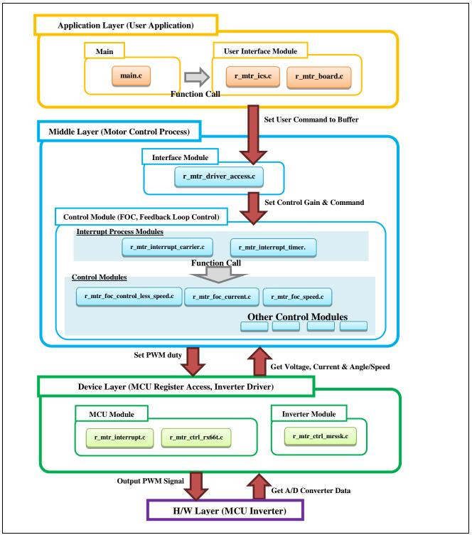
**Figure 2-3 Module Configuration**
