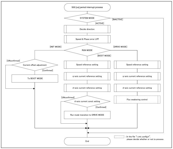
Figure 3-9 500[µs] Period Interrupt Process Flowchart
