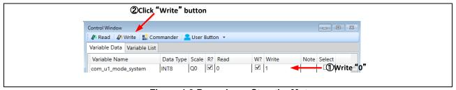
Figure 4-3 Procedure - Stop the Motor
