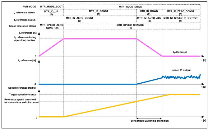
Figure 3-4 Startup Control of Sensorless Vector Control Software
