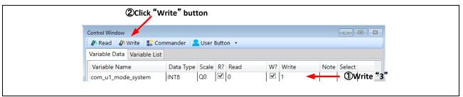
Figure 4-4 Procedure - Error Cancel Operation
