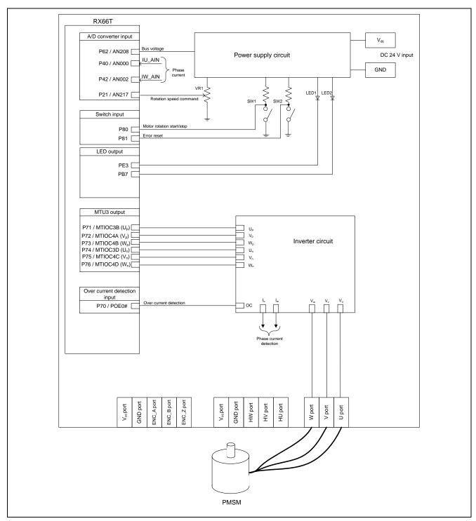
Figure 2-1 Hardware Configuration Diagram
