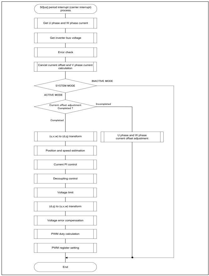
Figure 3-8 50[μs] Period Interrupt (Carrier Interrupt) Process Flowchart
