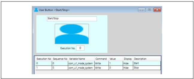
Figure 4-5 Driving or Stop the Motor
