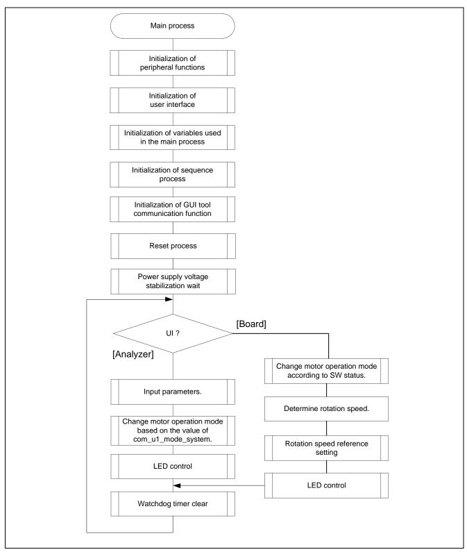
Figure 3-7 Main Process Flowchart
