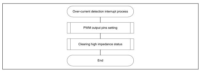
Figure 3-10 Over-Current Detection Interrupt Process Flowchart
