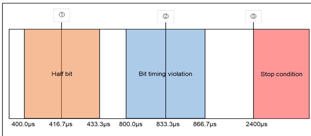
Figure 13 Multi-master Transmitter bit timing
