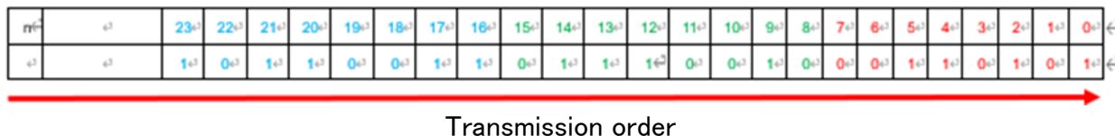
Figure 33 Example of transmission data arrangement
