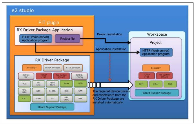
Figure 5.3.1 FIT Plugin Automatic Installation
