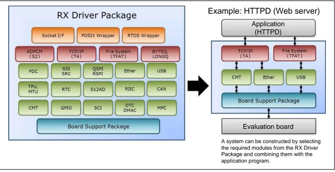
Figure 2.1.3 System Construction with the RX Driver Package
