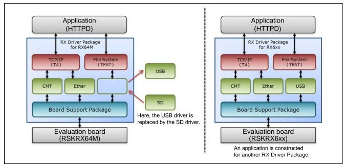
Figure 2.1.4 RX Driver Package Application Examples
