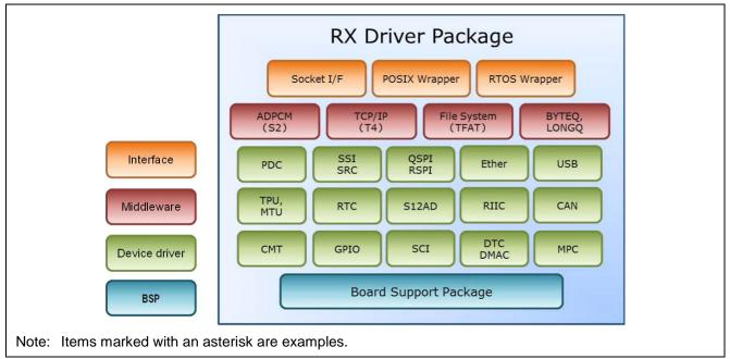
Figure 2.1.2 RX Driver Package Structure
