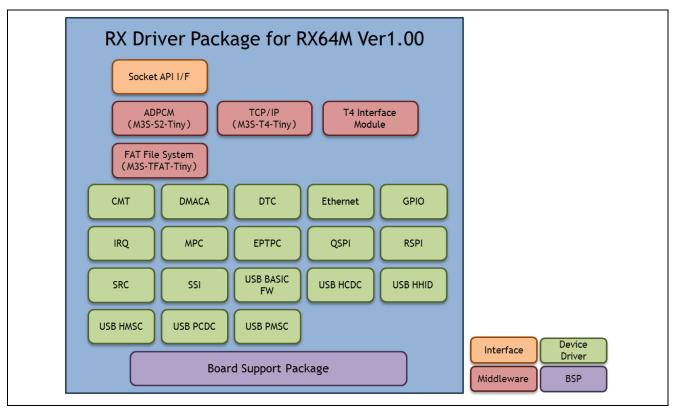
Figure 3.2.1 RX64M Group RX Driver Package FIT Module Structure
