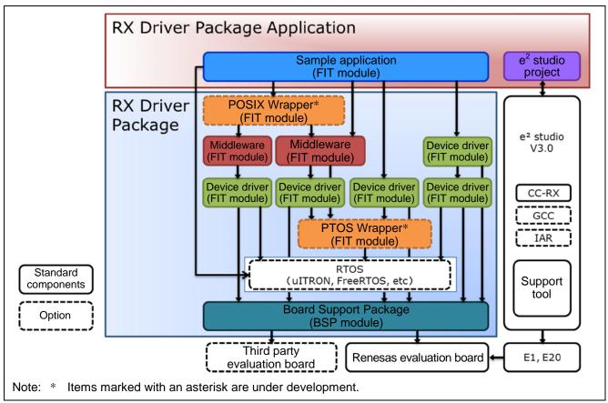
Figure 6.1 System Structure
