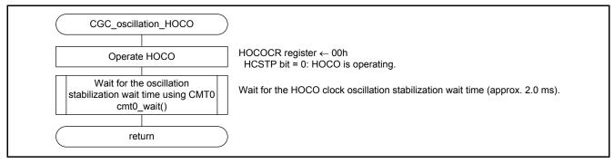
Figure 3.11 HOCO Clock Oscillation Setting
