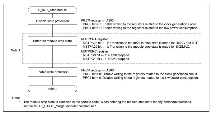
Figure 3.6 Stop Processing for Active Peripheral Functions after a Reset
