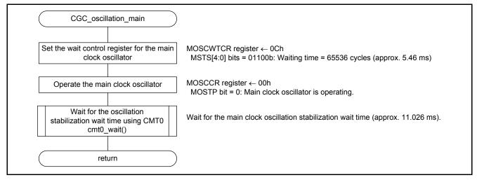
Figure 3.9 Main Clock Oscillation Setting
