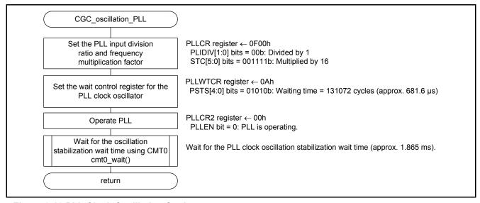
Figure 3.10 PLL Clock Oscillation Setting
