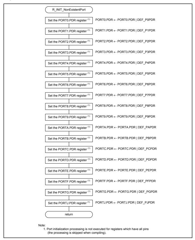
Figure 3.7 Nonexistent Port Initialization
