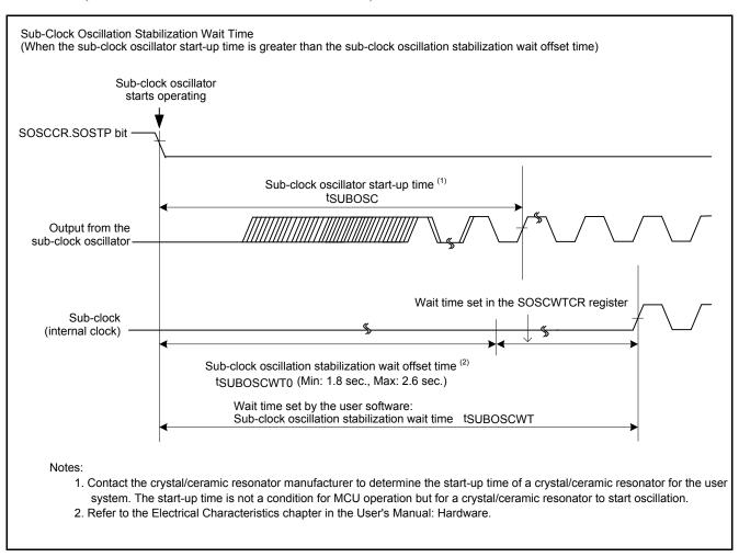
Figure 4.2 Sub-Clock Oscillation Stabilization Wait Time (when tSUBOSC is Greater than tSUBOSCWT0)
