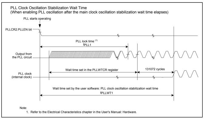
Figure 3.2 PLL Clock Oscillation Stabilization Wait Time
