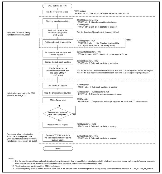
Figure 3.15 Sub-Clock Setting Pattern D (when the Sub-Clock is Used as the RTC Count Source and not Used as the System Clock)
