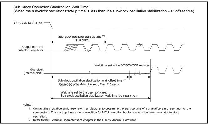
Figure 3.3 Sub-Clock Oscillation Stabilization Wait Time
