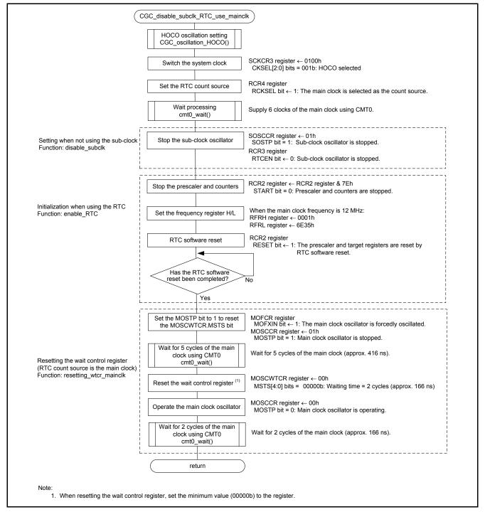
Figure 3.13 Sub-Clock Setting Pattern B (when the Sub-Clock is Stopped and the RTC Operates Using the Main Clock)
