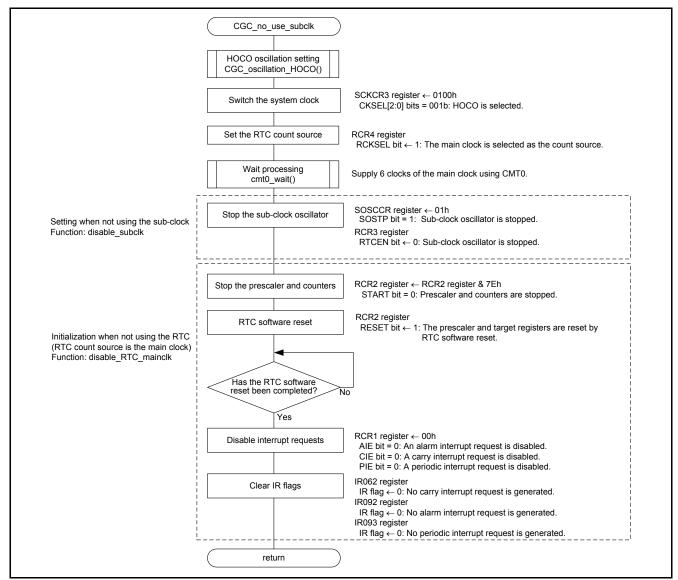
Figure 3.12 Sub-Clock Setting Pattern A (when the Sub-Clock is not Used as the System Clock or RTC Count Source)
