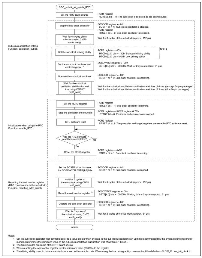
Figure 3.16 Sub-Clock Setting Pattern E (when the Sub-Clock is Used as Both the System Clock and RTC count source)
