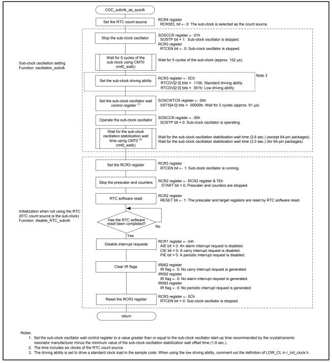
Figure 3.14 Sub-Clock Setting Pattern C (when the Sub-Clock is Used as the System Clock and not Used as the RTC Count Source)
