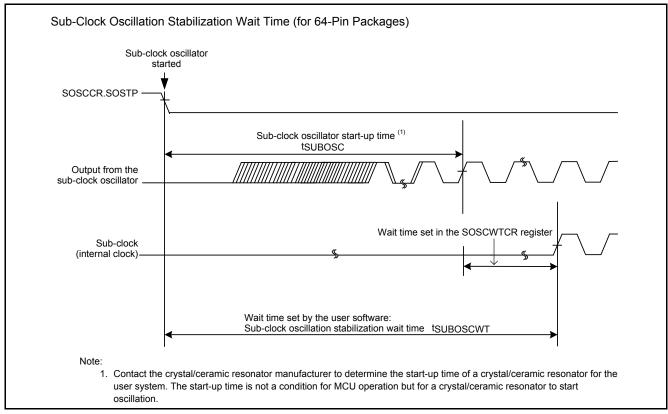
Figure 3.4 Sub-Clock Oscillation Stabilization Wait Time (for 64-Pin Packages)
