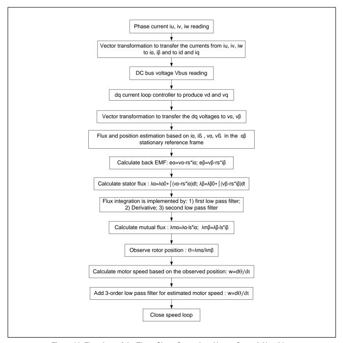
Figure 12 Flowchart of the Three-Shunt Sensorless Vector Control Algorithm
