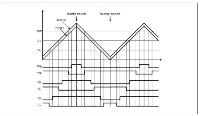
Figure 5 Three-Phase PWM Duties and PWM Waveform
