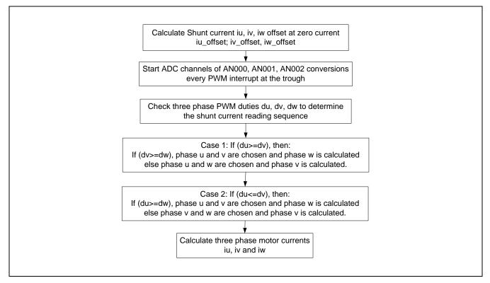
Figure 8 Flowchart of Three-Shunt Current Measurements
