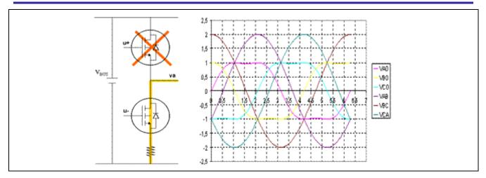
Figure 4 One Leg of the Inverter (Left) and Motor Voltage Waveforms (Right)
