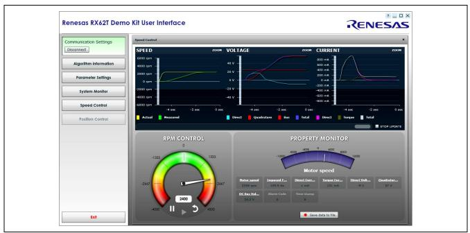
Figure 33 Setting the Speed to Turn the Motor in the GUI Application
