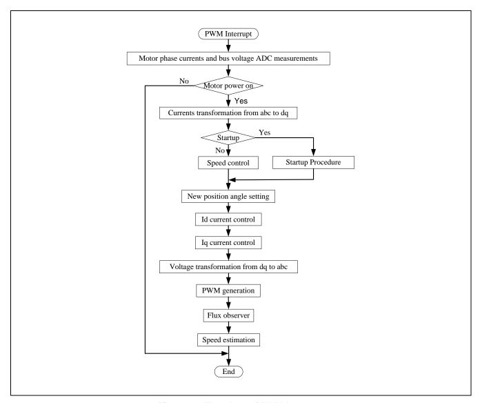
Figure 11 Flowchart of PWM Interrupt
