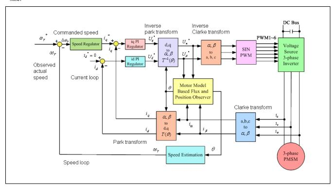
Figure 9 Block Diagram of Sensorless Vector Control
