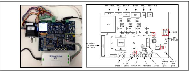
Figure 29 Running the Demo with e<sup>2</sup>studio and the GUI
