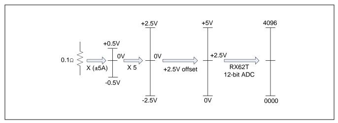
Figure 7 Motor Current Sensing Scale Translation
