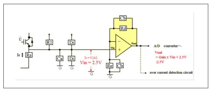
Figure 5 Motor Current Measurement with External Amplifier
