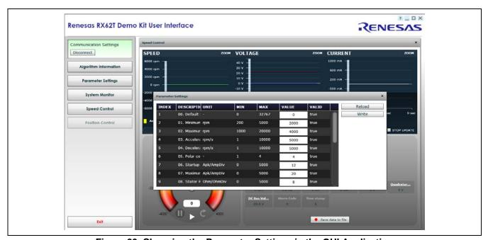
Figure 29 Changing the Parameter Settings in the GUI Application
