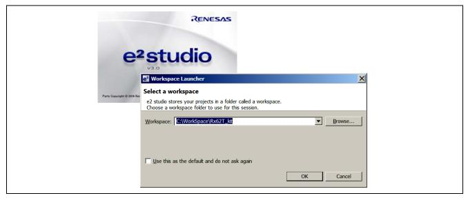
Figure 12 e<sup>2</sup> studio IDE Start-up Windows and Workspace Launcher
