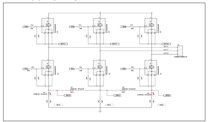
Figure 2 Single-Shunt Current Measurement in the Low Side Inverter Legs
