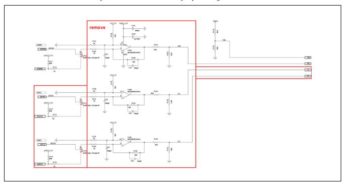
Figure 3 Single-Shunt Current Sampling with External Amplifier
