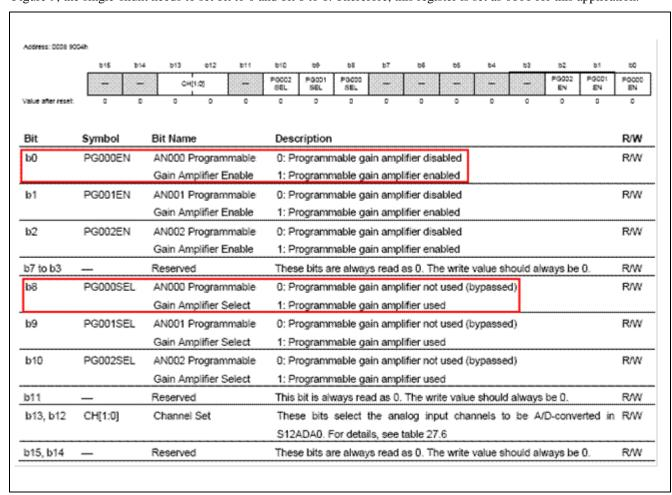
Figure 9 Bit Definition of the ADC Channel Select Register for Single-Shunt Current Measurement
