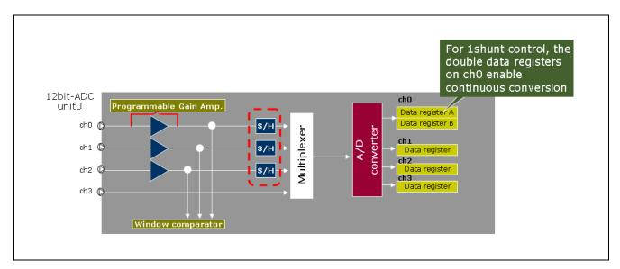
Figure 4 Structure of the RX62T ADC unit0 AN000 with PGA
