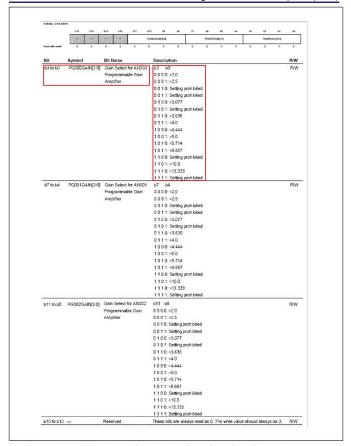
Figure 10 Bit Definition of the ADC PGA Register for the Single-Shunt Current Measurement
