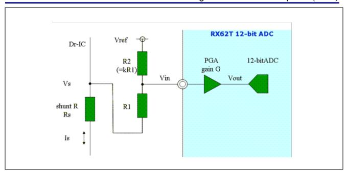
Figure 8 Shunt Current Sensing with PGA
