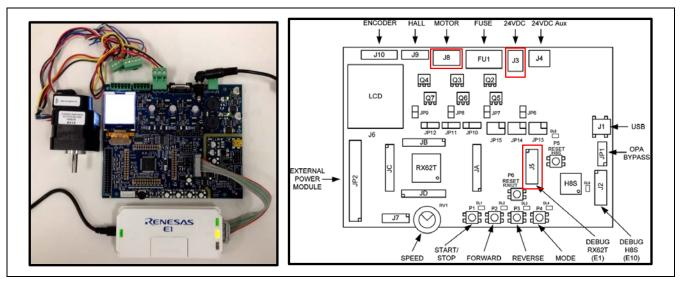
Figure 18 Debug Setup for the Demo Board
