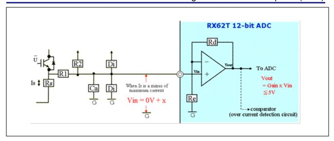
Figure 6 Motor Current Measurement with PGA
