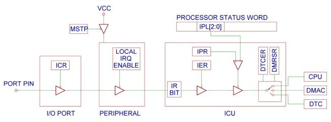
Figure 10.1 - RX Interrupt Flow
