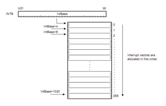
Figure 10.3 - Relocatable Vector Table
