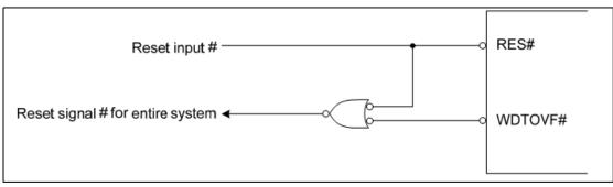
Figure 5.1 - Example of System Reset Circuit Using WDTOVF# Signal
