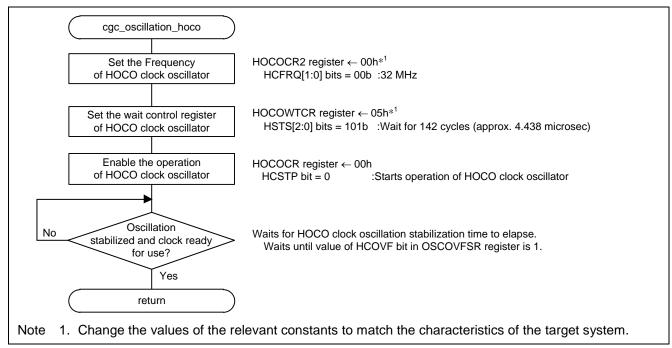
Figure 3.6 HOCO Clock Oscillation Enable
