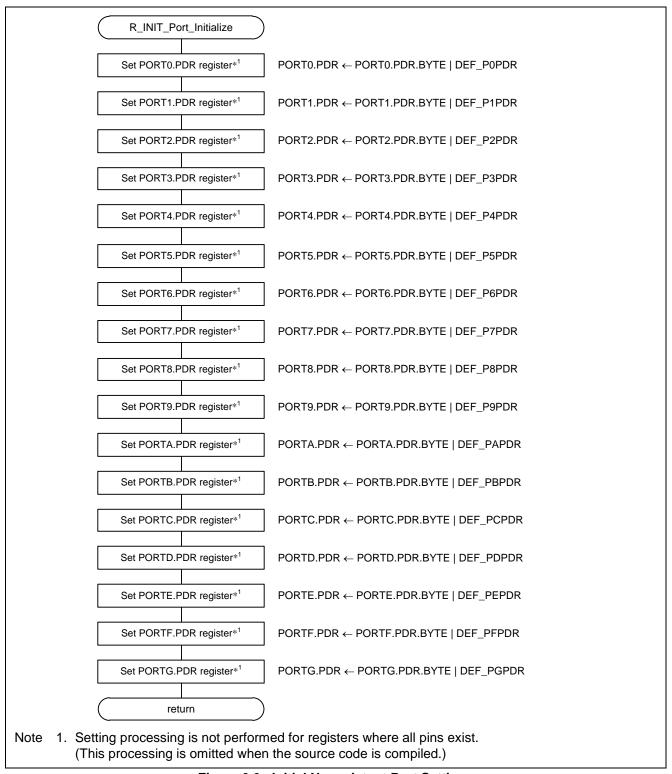
Figure 3.3 Initial Nonexistent Port Settings
