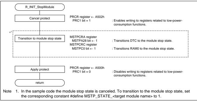
Figure 3.2 Disable Peripheral Modules Still Running After a Reset
