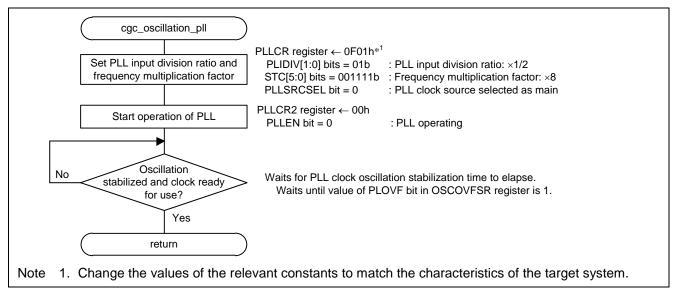
Figure 3.7 PLL Clock Oscillation Enable
