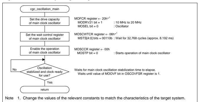
Figure 3.5 Main Clock Oscillation Enable
