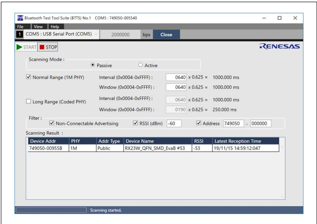
Figure 3-5. Scanning setting (receiving device side)
