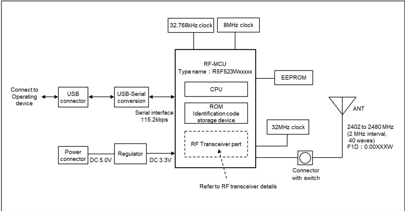
**Figure 2-1. Block diagram of radio equipment (Example)**
