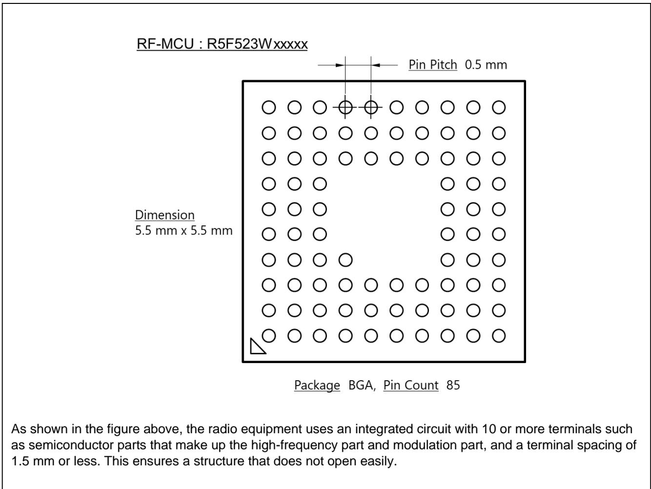
**Figure 2-4. Dimensions and outline drawing of shape (Example)**
