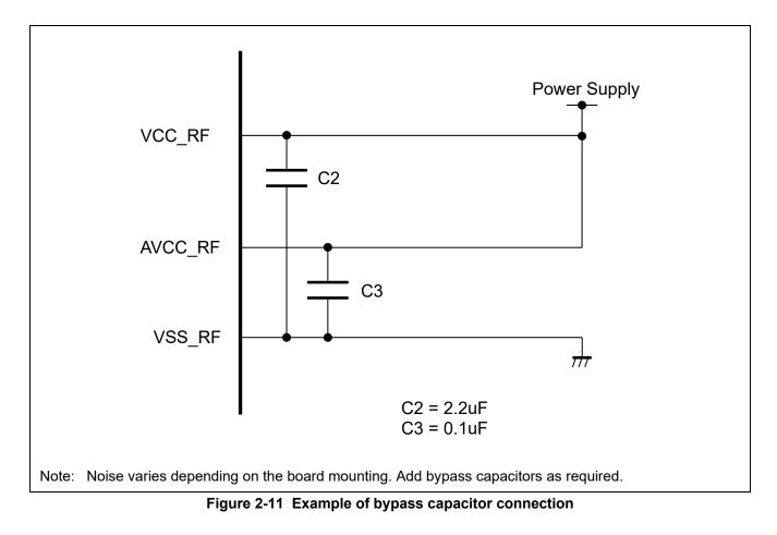
Figure 2-11 shows an example of how to place the bypass capacitors.
