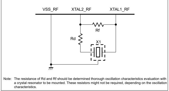
Figure 2-1 Example of the crystal resonator connection.
