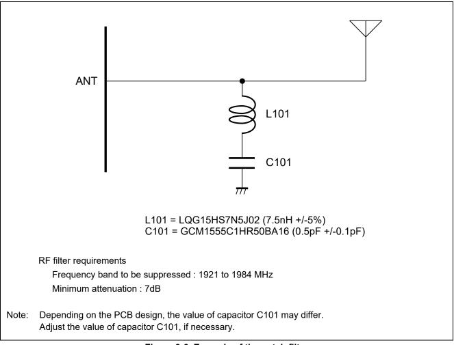
Figure 3-6 Example of the notch filter
