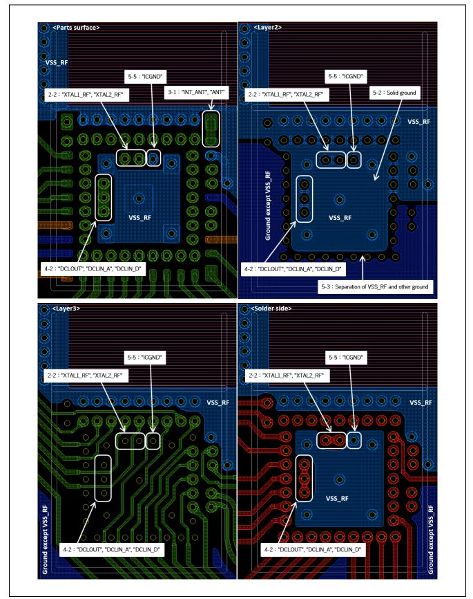
Figure 4-3 Example of the pattern under the RX23W LGA package
