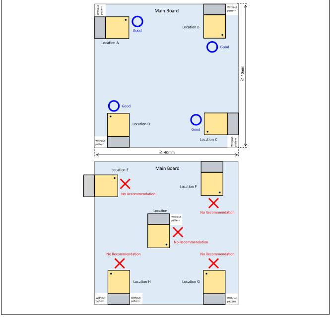
Figure 4-6 Example of the main board layout
