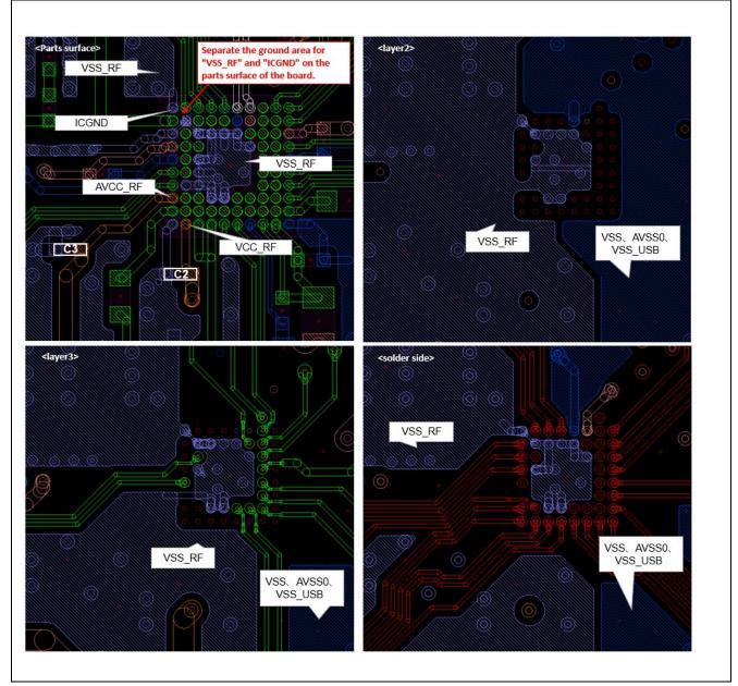
Figure 3-12 Example of the ground pattern
