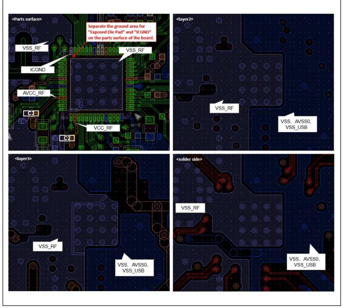
Figure 2-12 Example of the ground pattern
