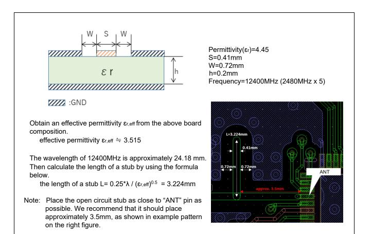
Figure 2-4 Example of the open circuit stub
