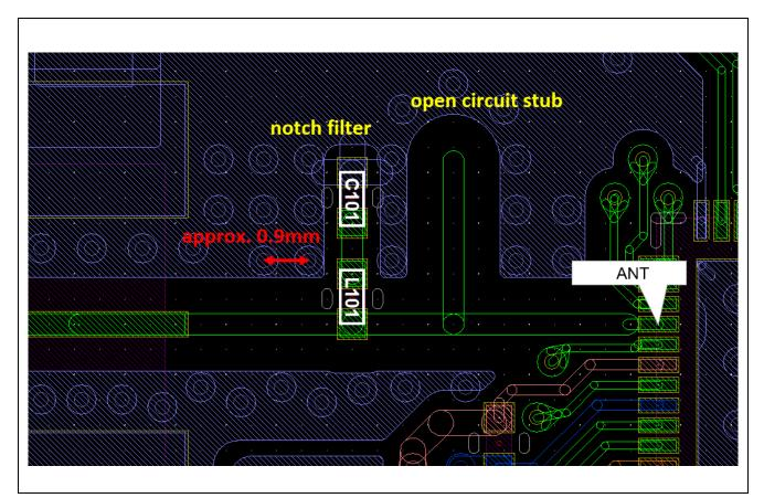
Figure 2-3 shows an example of the pattern around "ANT" pin.
