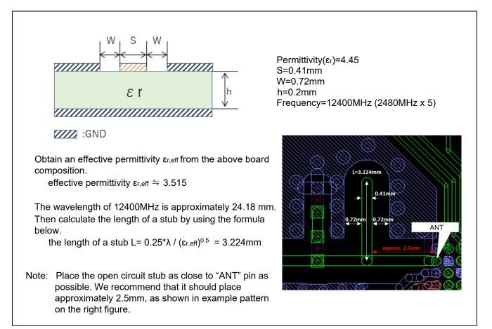
Figure 3-4 Example of the open circuit stub
