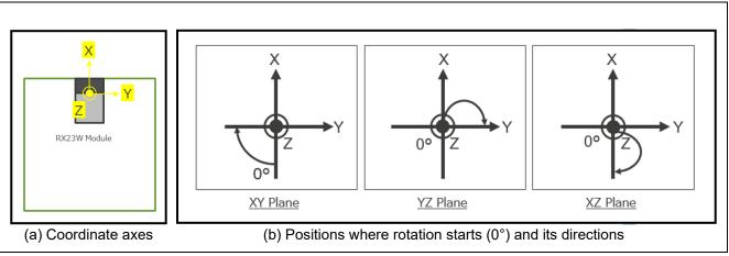
Figure 4-7 Coordinates and Rotation of the main board
