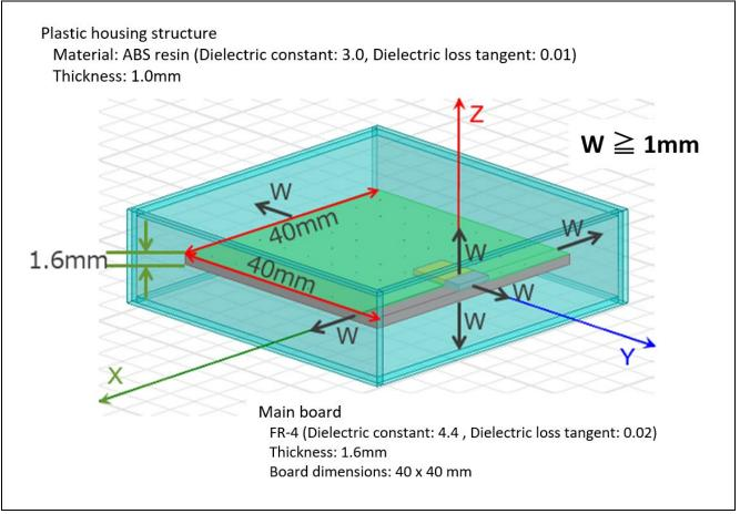
Figure 4-9 Plastic housing conditions
