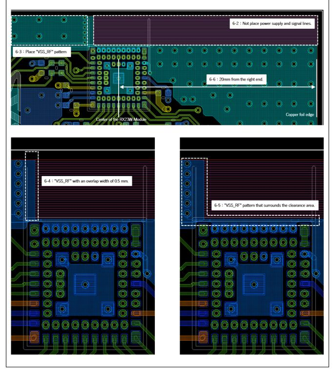
Figure 4-5 Example of the antenna layout
