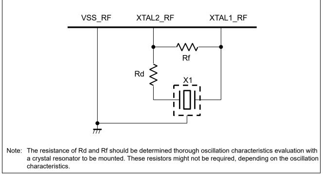
Figure 3-1 Example of the crystal resonator connection.
