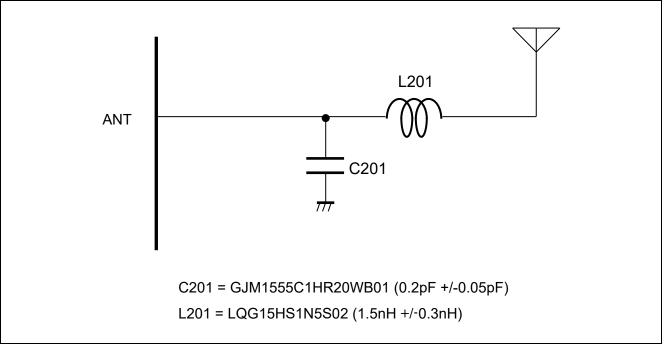
Figure 2-5 Example of LPF using SMD parts
