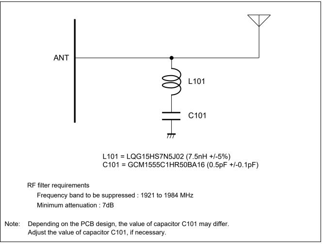
Figure 2-6 Example of the notch filter
