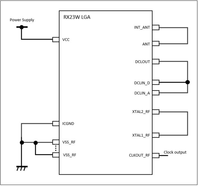
Figure 4-1 Example of connections for each pin
