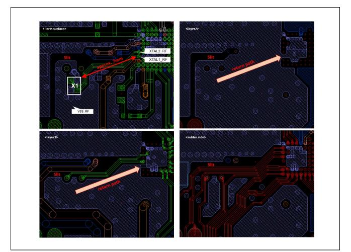
Figure 3-2 Example of the pattern around the crystal resonator
