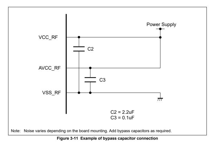
Figure 3-11 shows an example of how to place the bypass capacitors.
