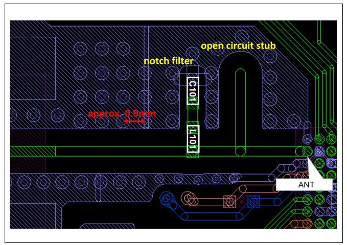
Figure 3-3 Example of the pattern around "ANT" pin
