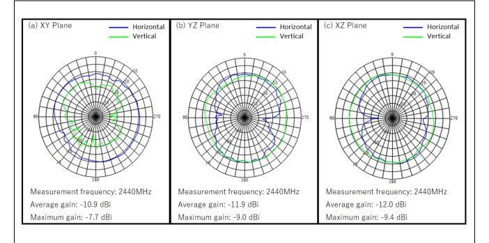
Figure 4-8 Measurement results of the internal antenna emission characteristics
