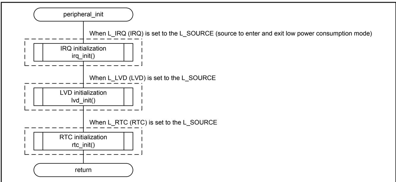
Figure 5.8 Peripheral Function Initialization
