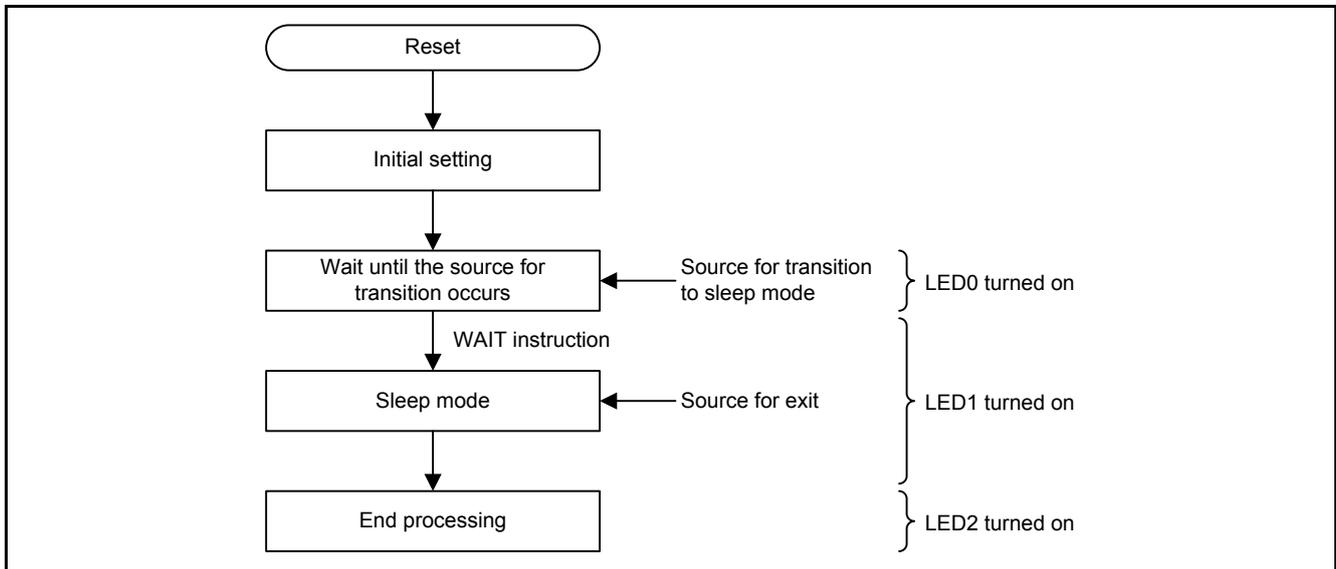
Figure 5.1 Operation Overview when Entering and Exiting Sleep Mode
