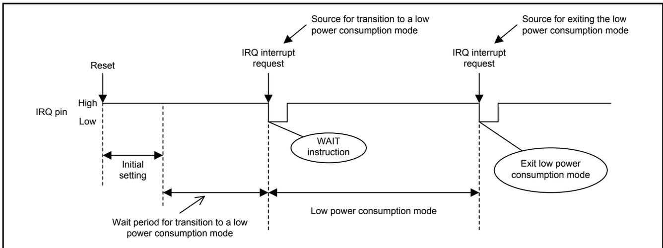
Figure 5.3 Timing for Entering and Exiting a Low Power Consumption Mode Using the IRQ
