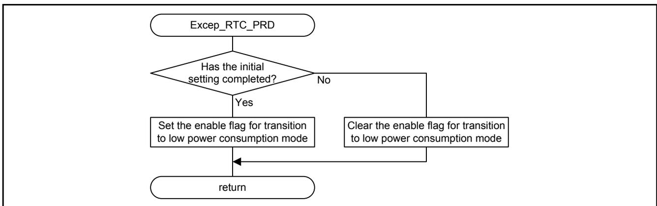
Figure 5.18 RTC.PRD Interrupt Handling
