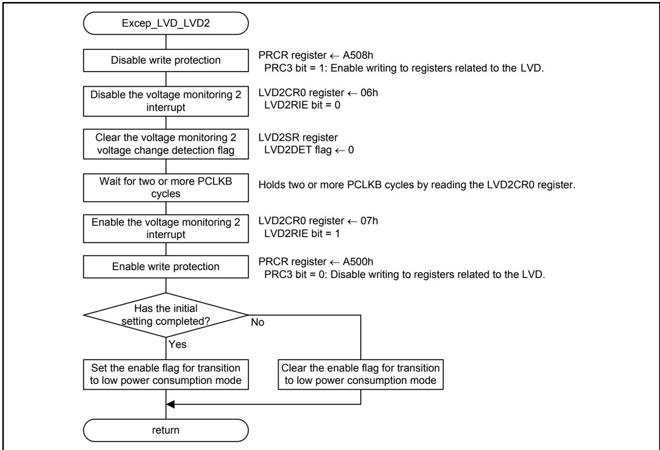
Figure 5.17 LVD2 Interrupt Handling
