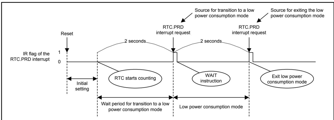
Figure 5.4 Timing of Entering and Exiting a Low Power Consumption Mode Using the RTC
