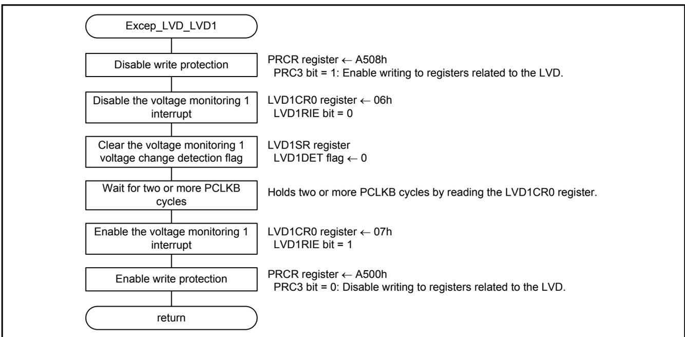
Figure 5.16 LVD1 Interrupt Handling
