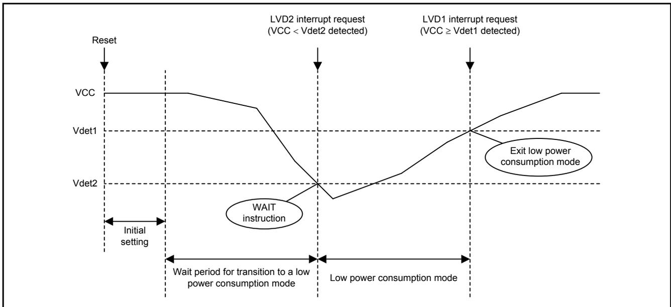
Figure 5.5 Timing of Entering and Exiting a Low Power Consumption Mode Using the LVD
