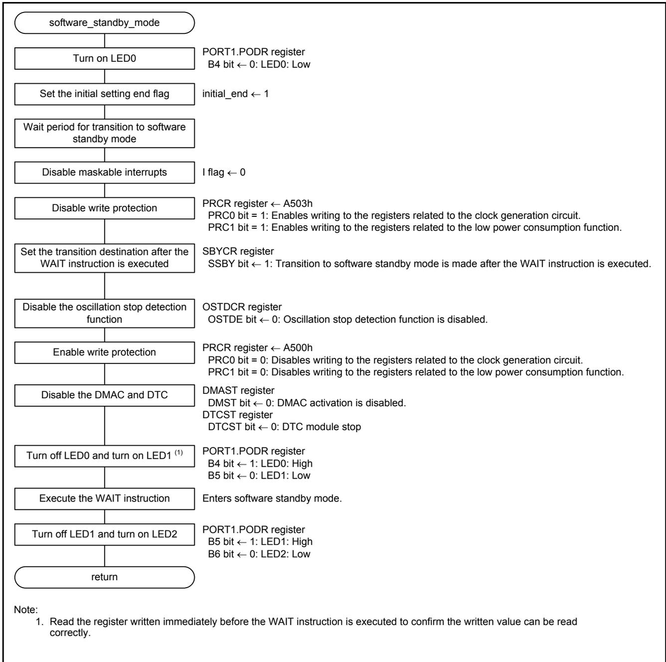
Figure 5.10 Transition to Software Standby Mode
