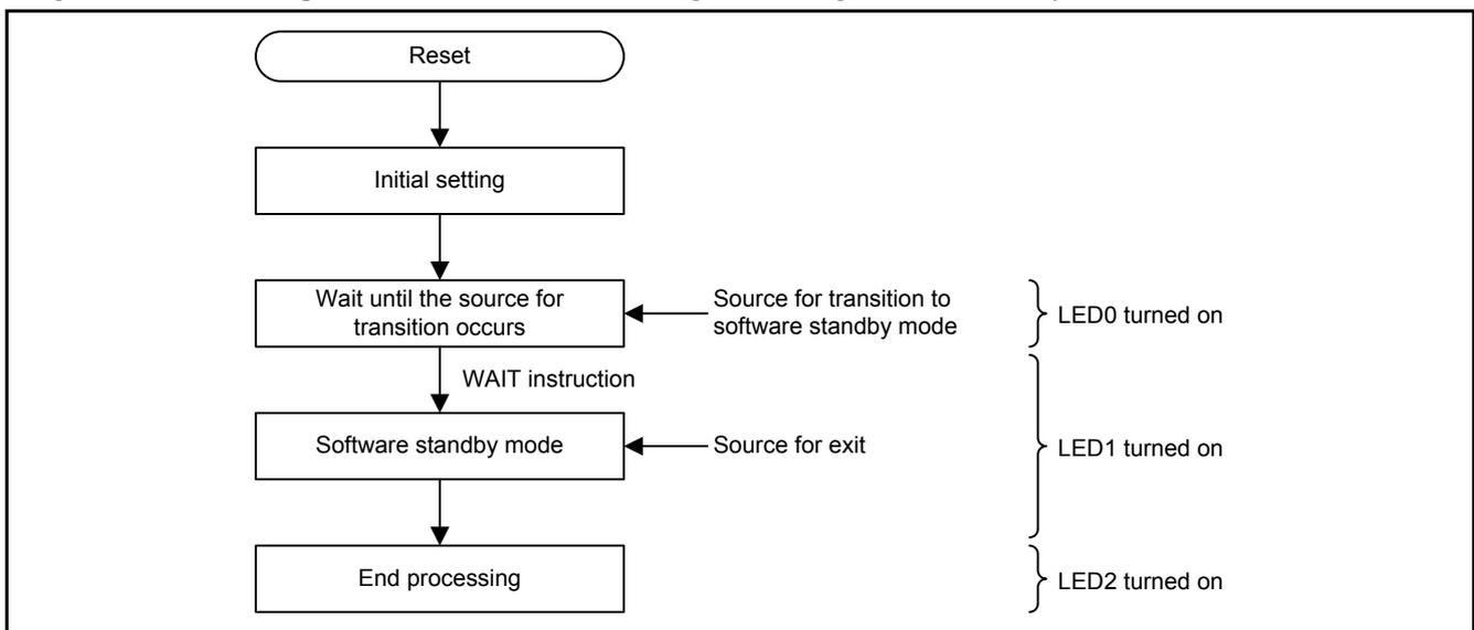
Figure 5.2 Operation Overview when Entering and Exiting Software Standby Mode
