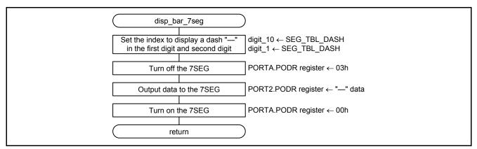
Figure 5.9 Processing to Display a Dash on the 7SEG
