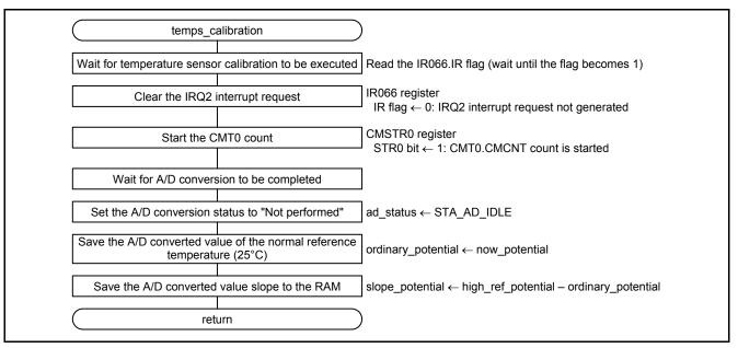
Figure 5.15 Processing for Temperature Sensor Calibration
