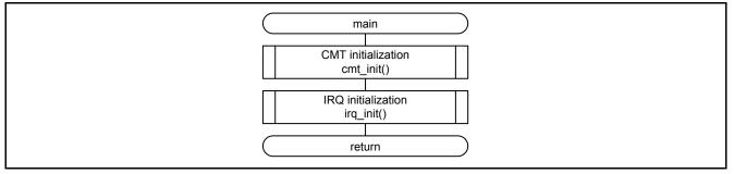
Figure 5.4 Peripheral Function Initialization
