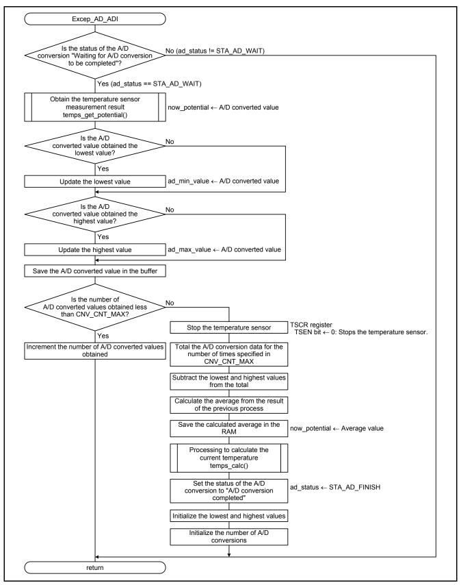
Figure 5.18 A/D Conversion Complete Interrupt Handling
