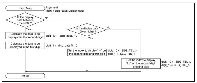
Figure 5.7 Processing to Update the 7SEG Display Data
