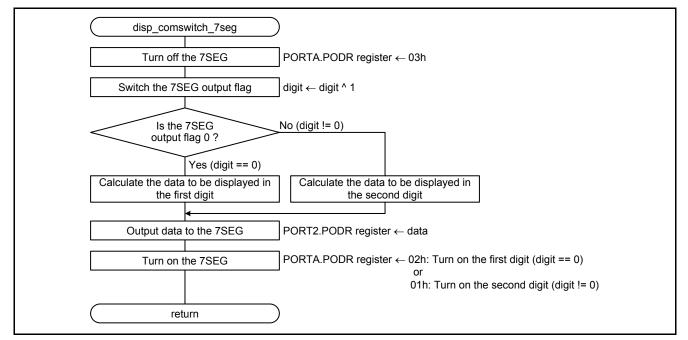
Figure 5.8 Processing to Switch the 7SEG Select Output
