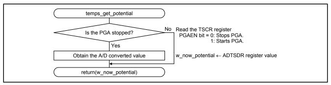
Figure 5.13 Obtain the Temperature Sensor Measurement Result
