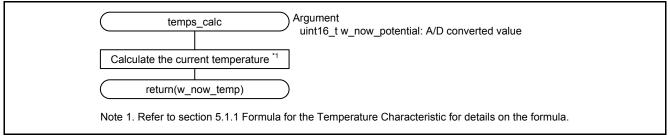
Figure 5.17 Processing to Calculate the Current Temperature
