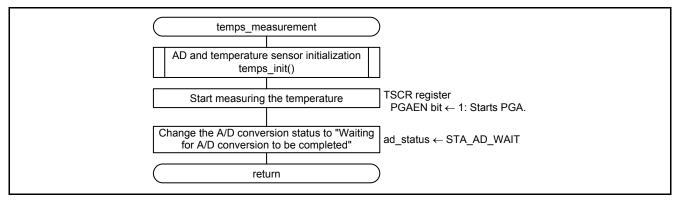
Figure 5.16 Processing for Temperature Sensor Measurement
