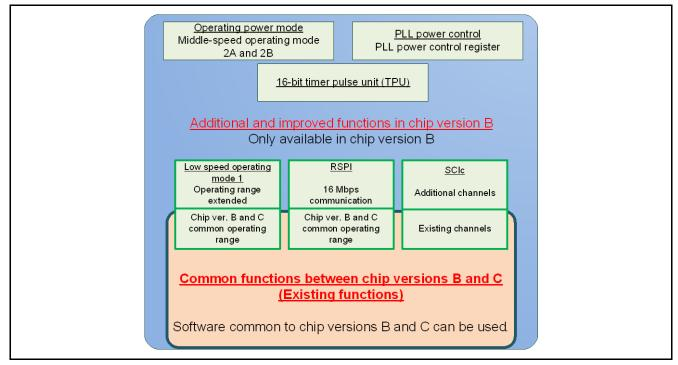
Figure 2.1 Software Compatibility Between Chip Versions B and C
