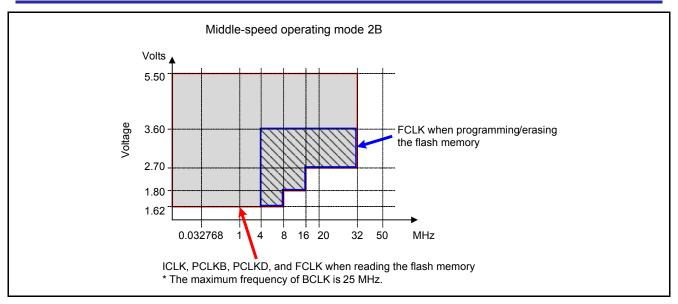
Figure 2.3 Operating Frequency and Operating Voltage Ranges in Middle-Speed Operating Mode 2B
