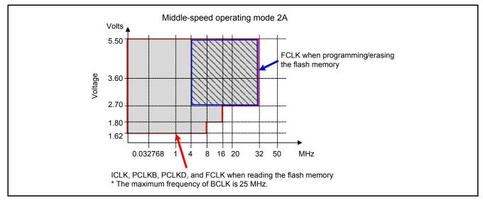
Figure 2.2 Operating Frequency and Operating Voltage Ranges in Middle-Speed Operating Mode 2A
