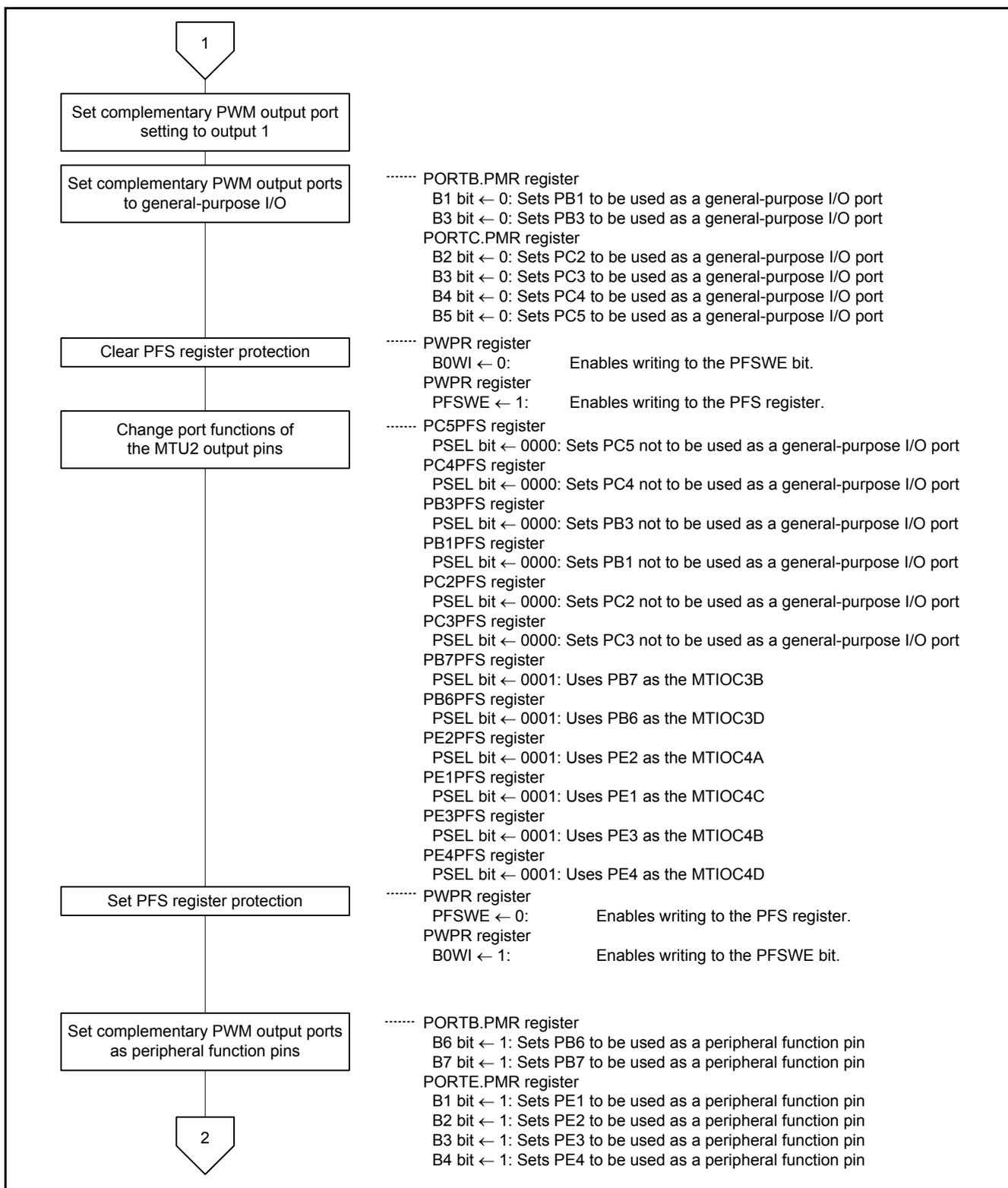
Figure 5.11 Complementary PWM Output Port Switching (2/2)
