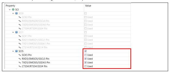
In the pin configuration screen, the assignment is changed to PA3 for RXD5 and PA4 for TXD5.
