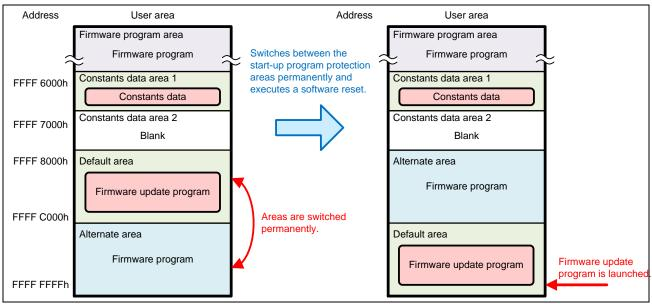
Figure 5.15 Firmware Program Operation (for RX231 Group)
