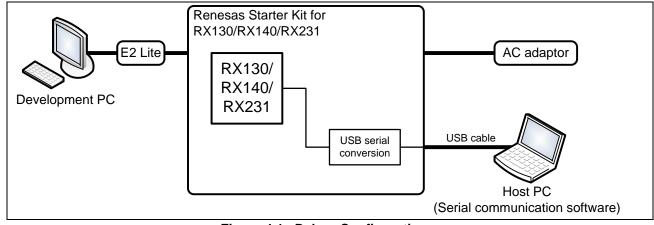
Figure 4.1 Debug Configuration
