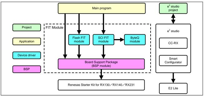
Figure 1.2 Module Configuration
