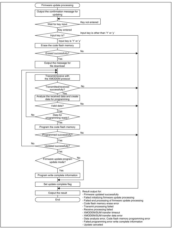
Figure 5.31 Flowchart of Firmware Update Processing
