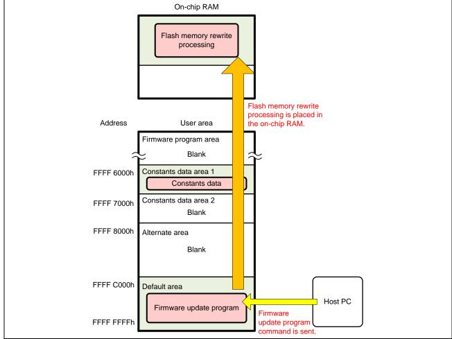
Figure 5.3 Sending the Firmware Program Update Command (for RX231 Group)
