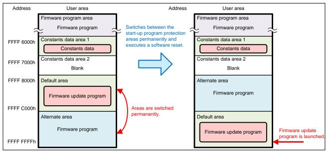
Figure 5.8 Operation of the Firmware Program Before Being Updated (for RX231 Group)
