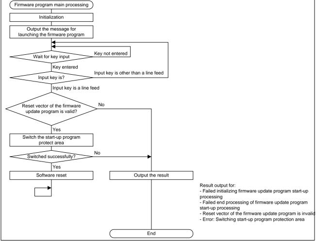
Figure 5.43 Flowchart of the Firmware Program
