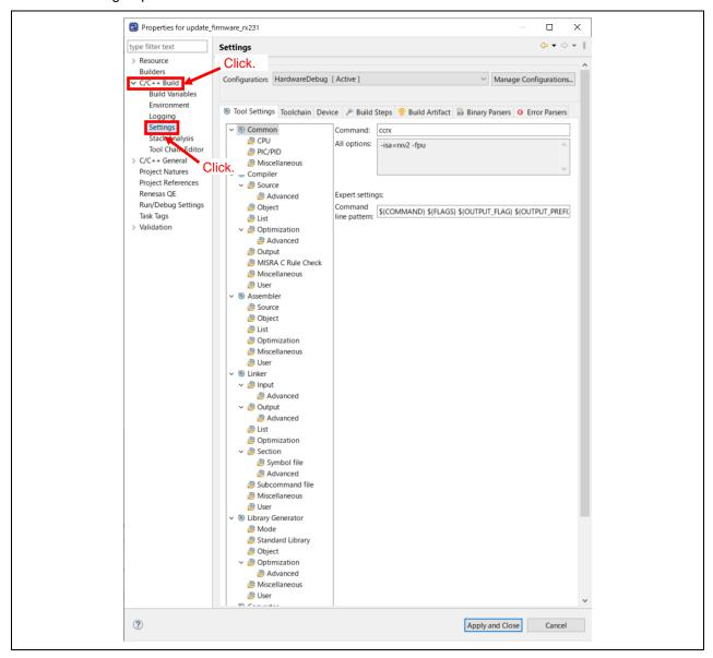
3. In the Tool Settings tab, confirm that settings have been changed to values described in Table 3.1, Table 3.2 and Table 3.3 for the firmware update project and the firmware project, respectively.
