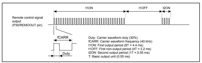
Figure 1.1 Remote Control Signal Output
