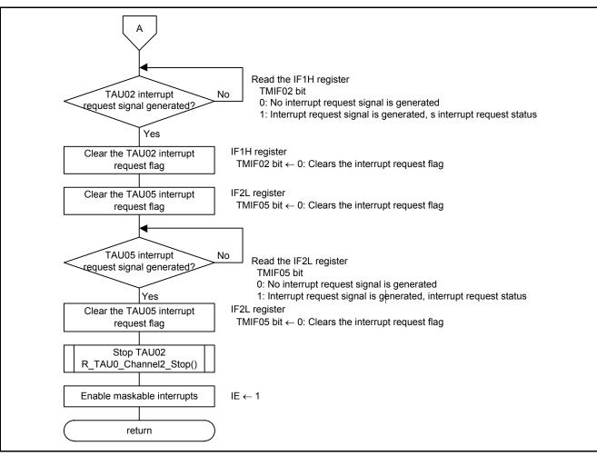
Figure 4.15 Remote Control Output Control Setting (2/2)
