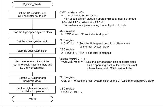
Figure 4.5 CPU Clock Initialization
