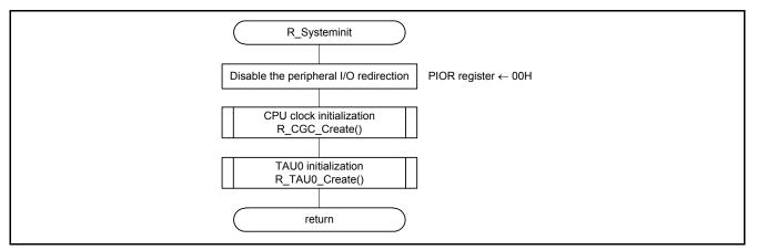
**Figure 4.4 Peripheral Function Initialization**
