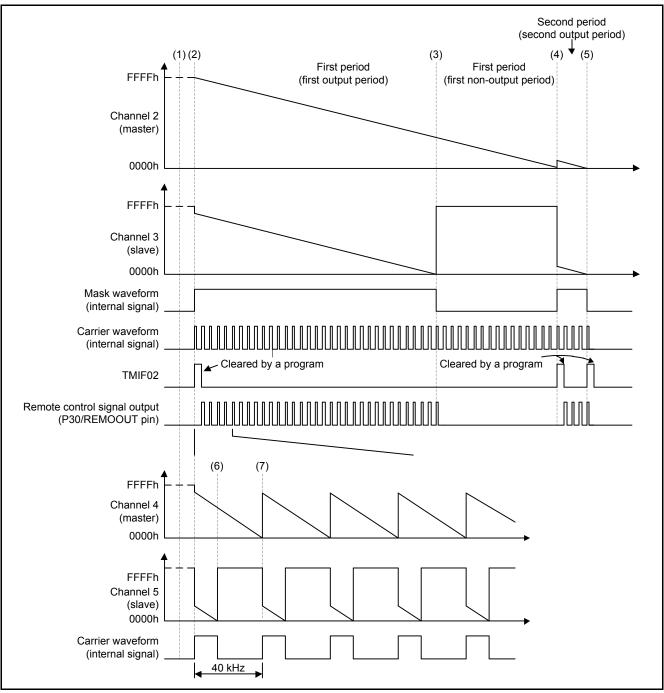
Figure 4.1 Behavior of Remote Control Output
