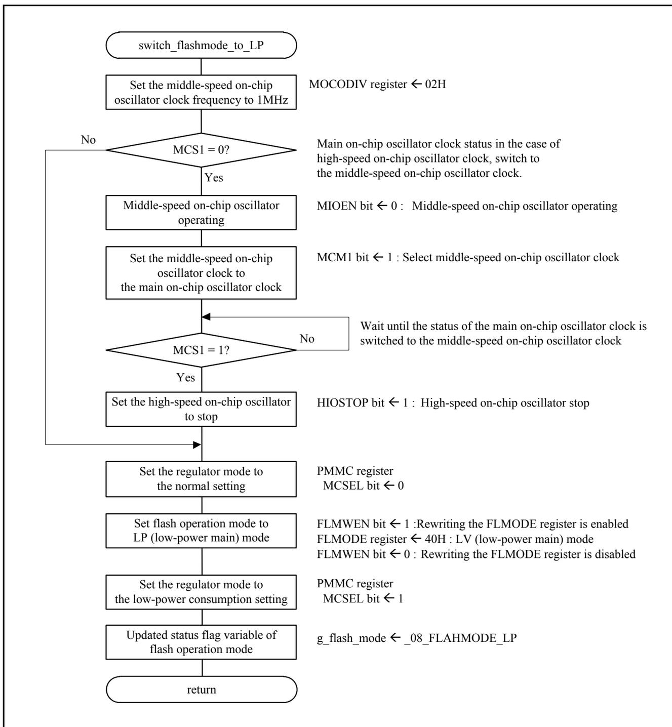
Figure 4.23 Flash operation mode switching (LP normal) processing
