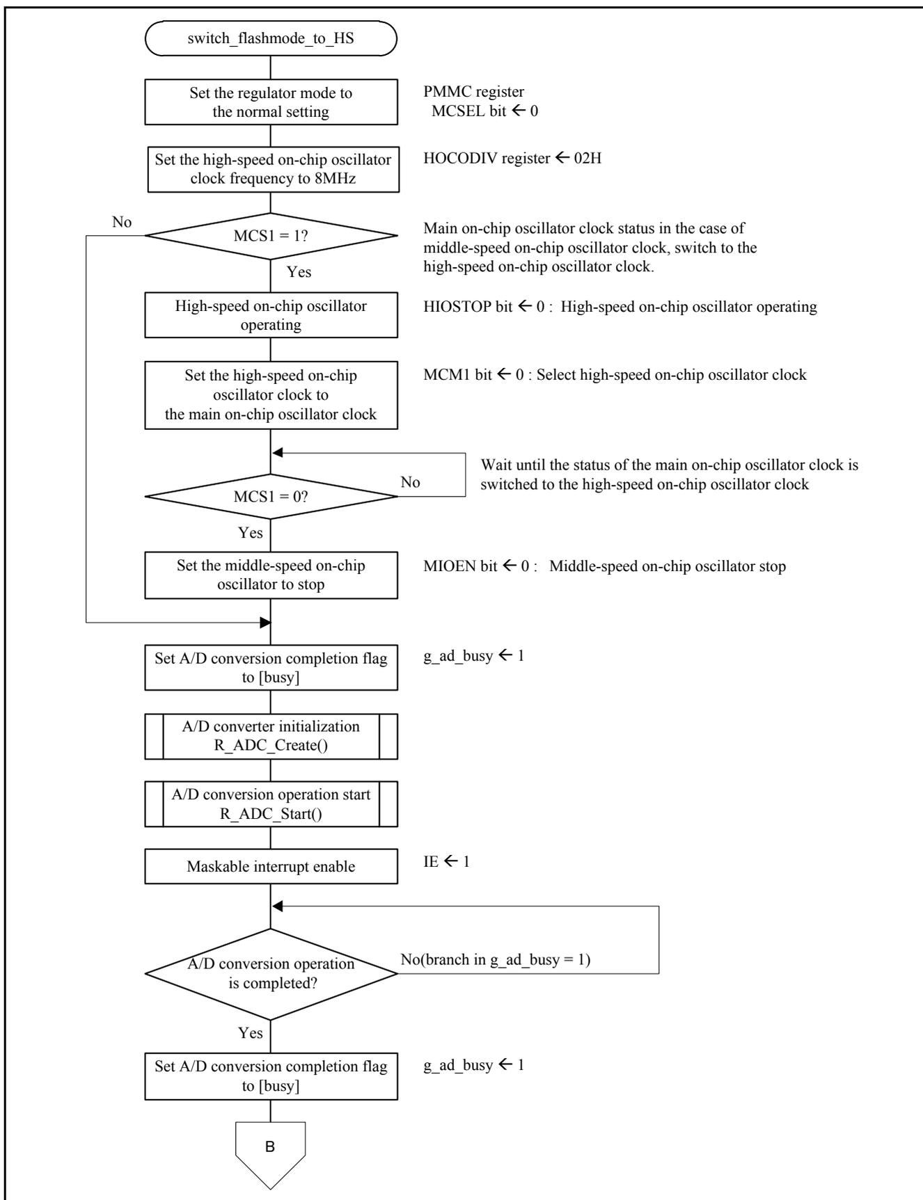
Figure 4.18 Flash operation mode switching (HS) processing(1/2)
