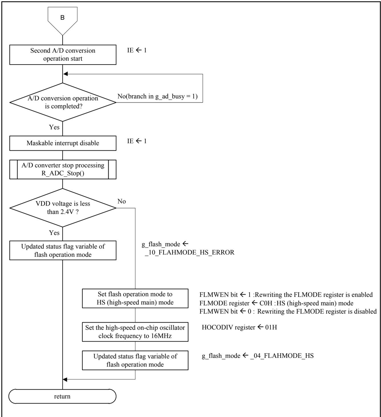
Figure 4.19 Flash operation mode switching (HS) processing(2/2)
