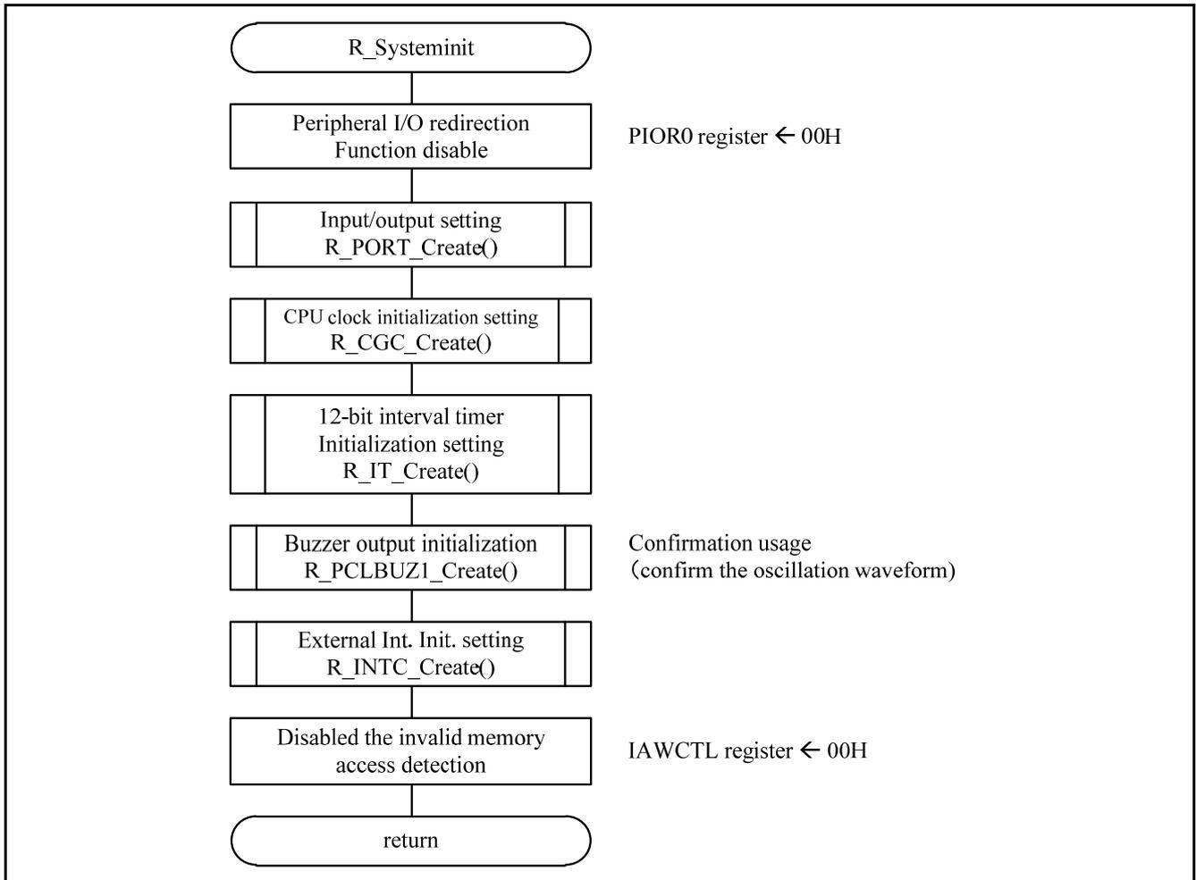
Figure 4.3 Peripheral function initialization
