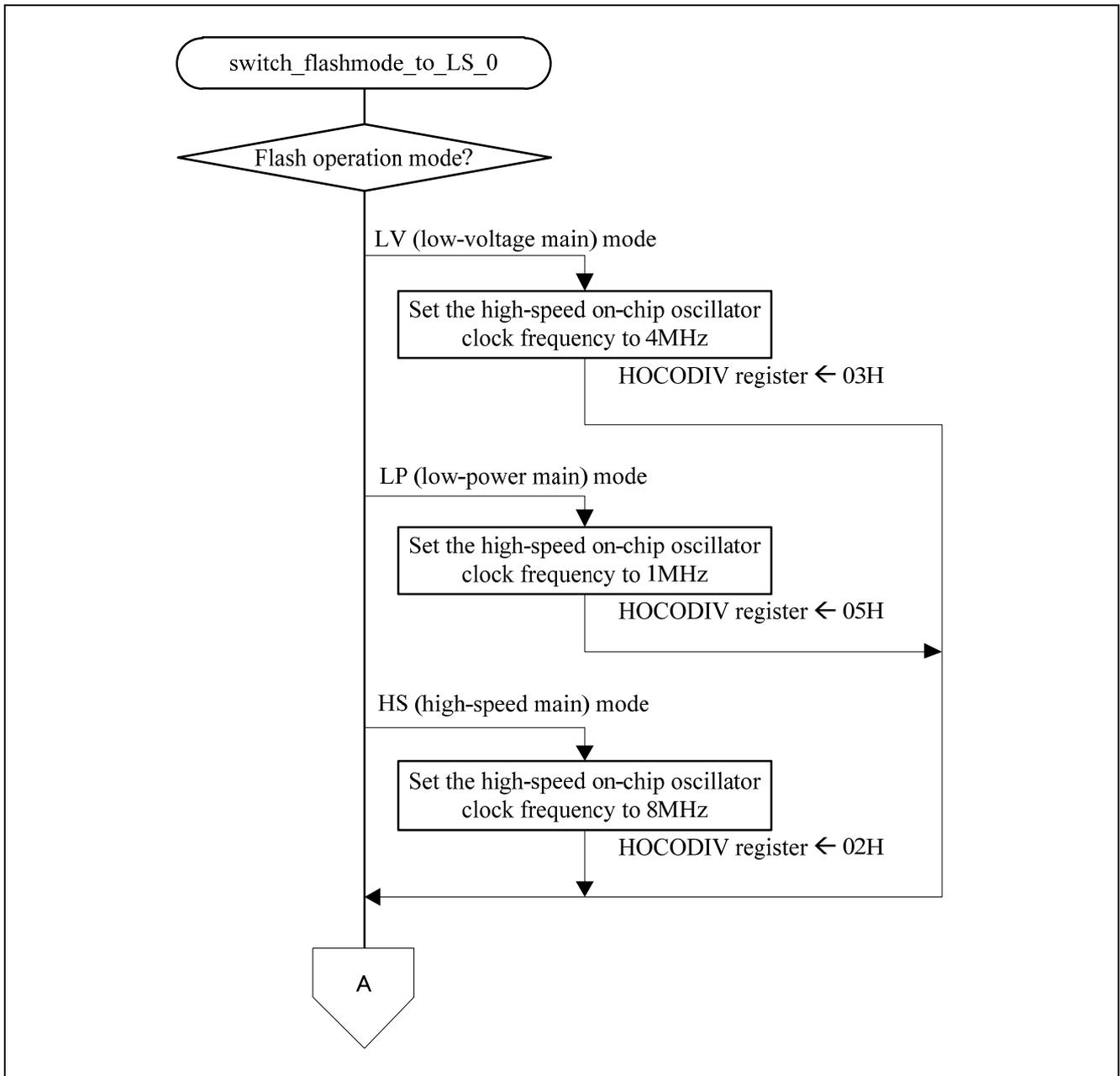
Figure 4.15 Flash operation mode switching (LS normal) processing(1/2)
