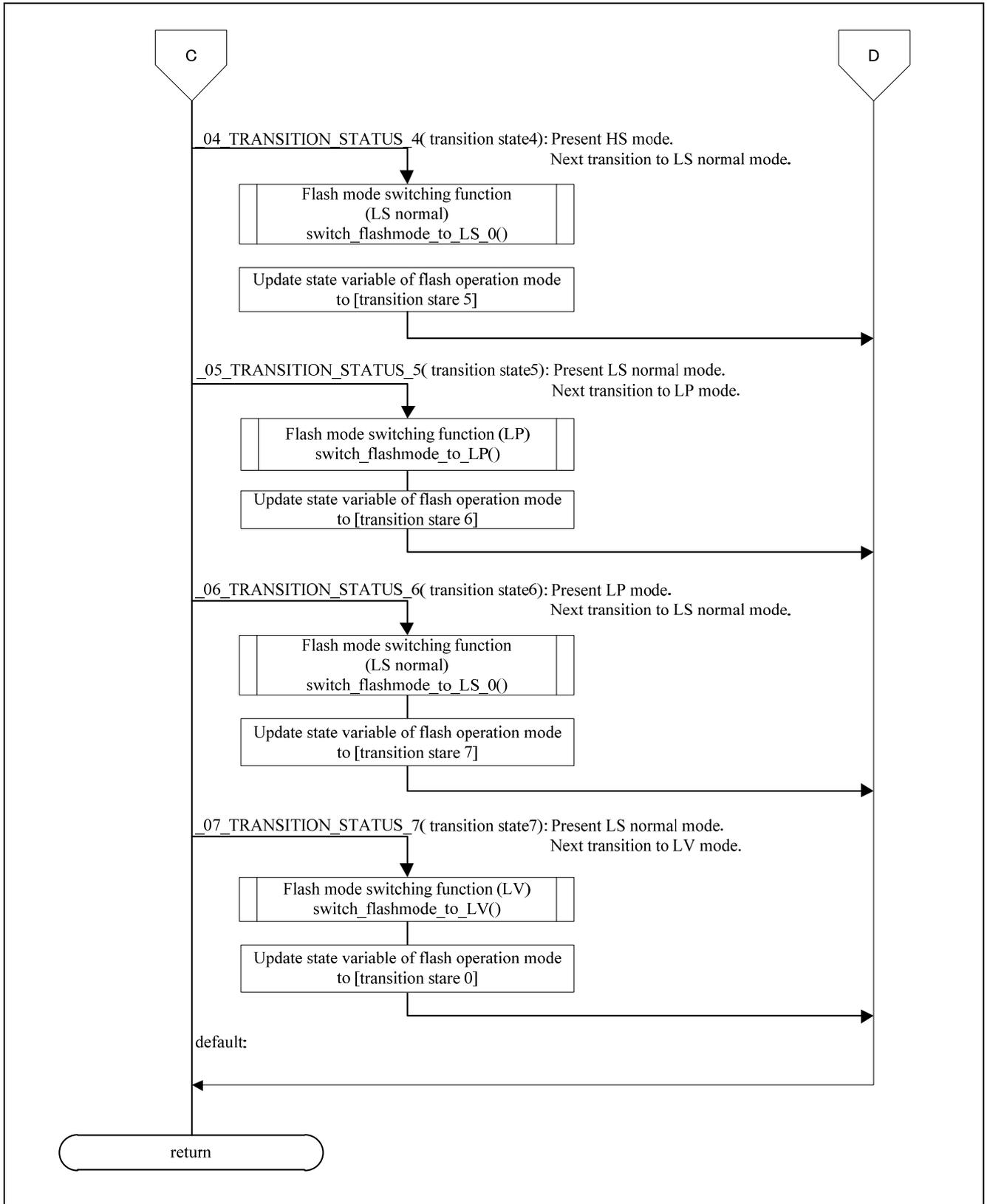
Figure 4.25 External interrupt (INTP0) processing(2/2)
