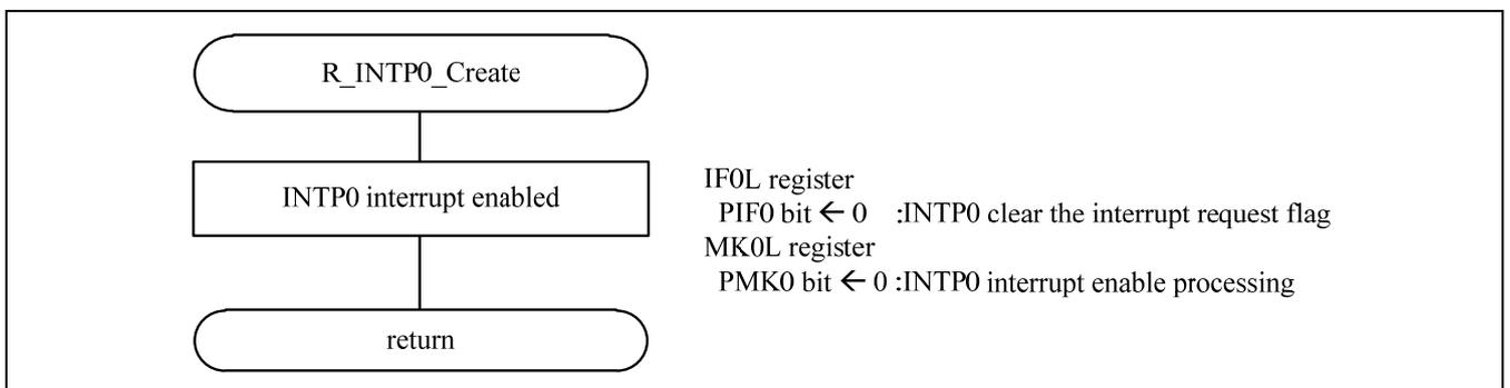
Figure 4.11 INTP0 interrupt enable processing
