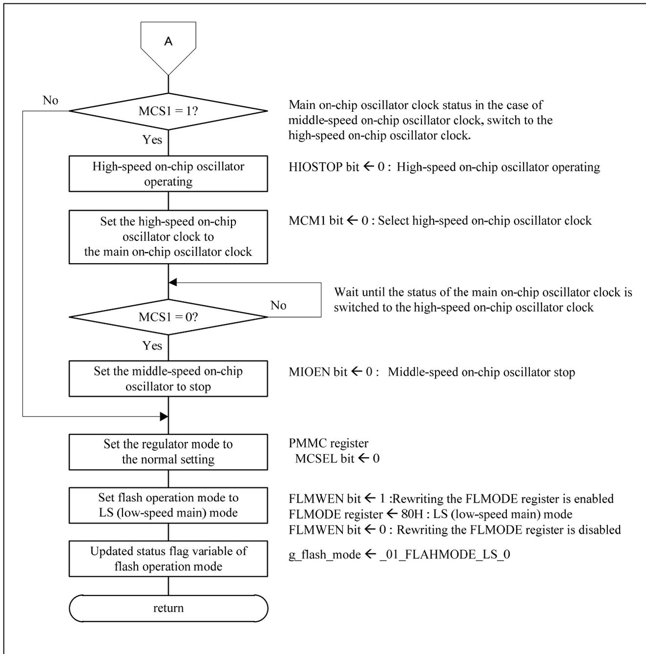
Figure 4.16 Flash operation mode switching (LS normal) processing(2/2)
