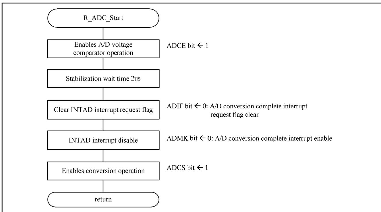
Figure 4.21 A/D conversion operation start processing
