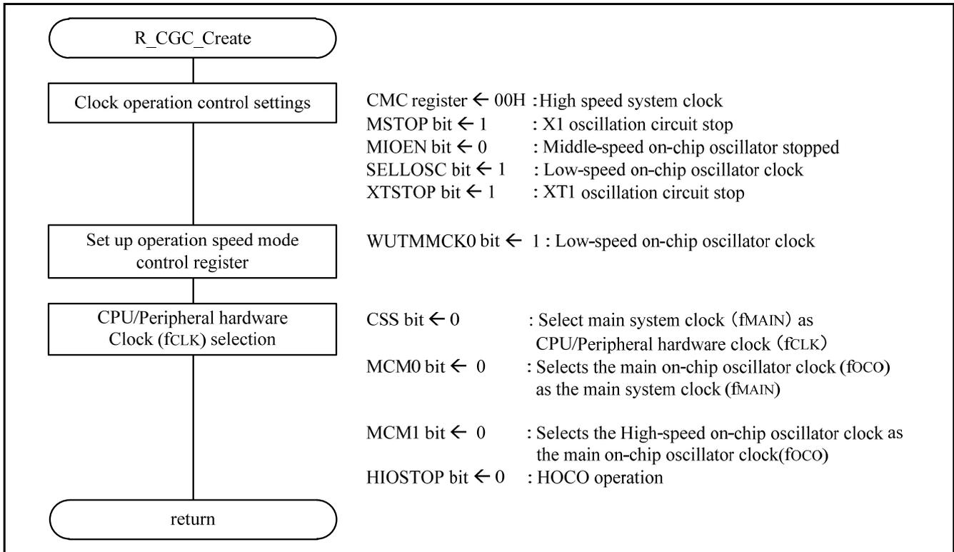
Figure 4.5 CPU clock initialization
