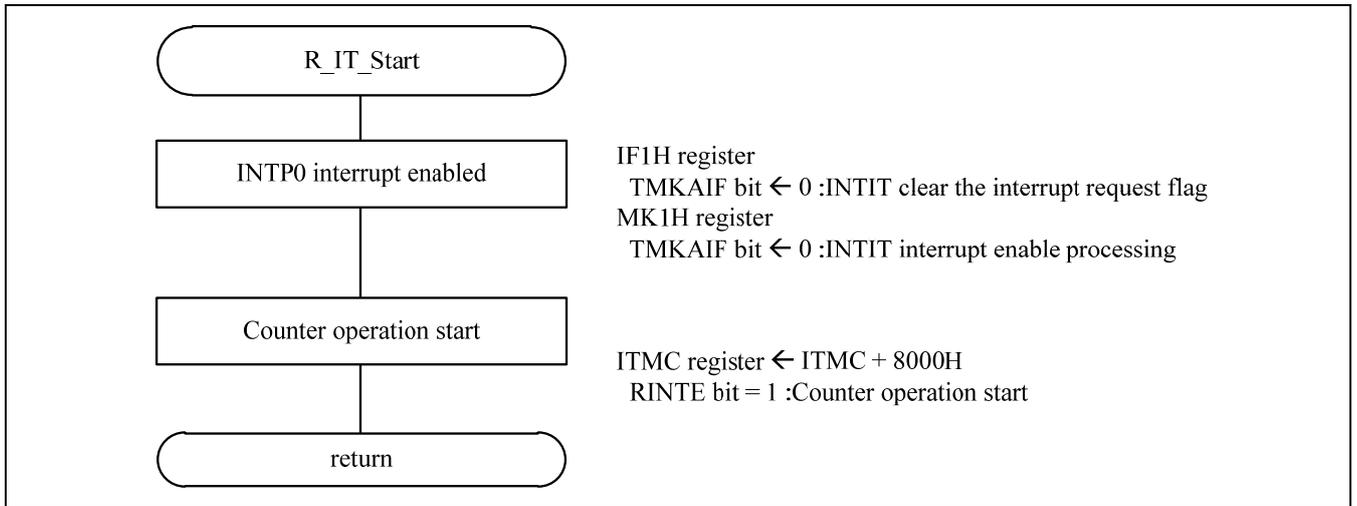
Figure 4.12 12-bit interval timer start processing
