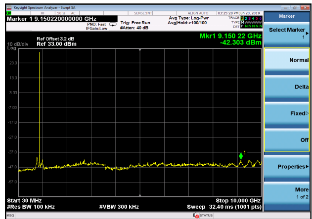
Figure 13 TX Spurious emission ( V_{DDPA} = 4.0\text{ V} , V_{DD} = V_{DDRF} = 3.3\text{ V} , 50kbps, mod index = 1, Frequency = 915.0 MHz, Gain Setting = 90, Temperature = Room)
