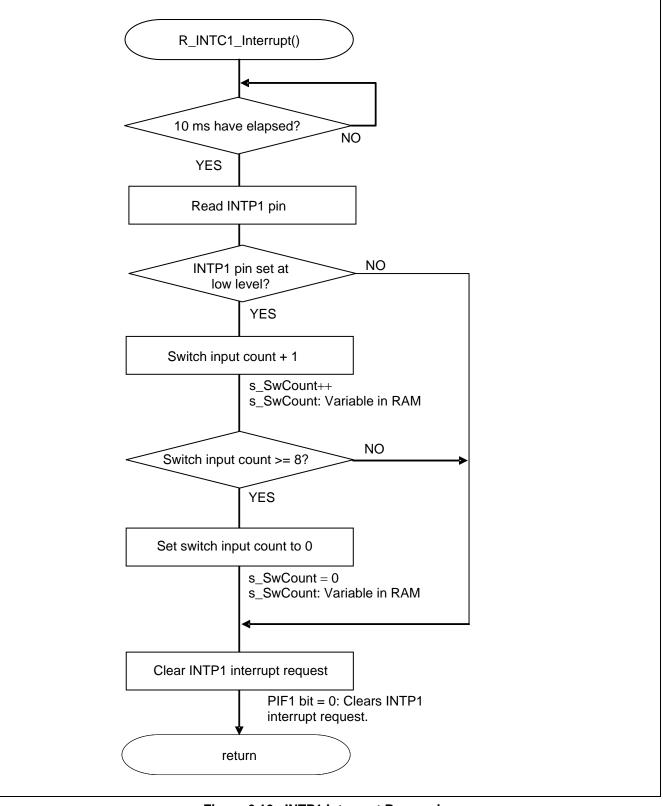
Figure 6.10 INTP1 Interrupt Processing
