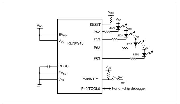
Figure 5.1 Hardware Configuration
