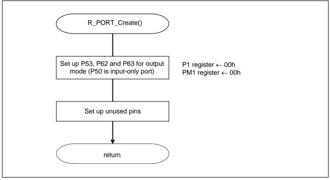
Figure 6.5 I/O Port Setup
