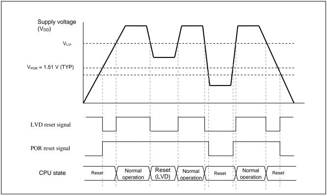
Figure 2.1 Overview of LVD Operation (Reset Mode)
