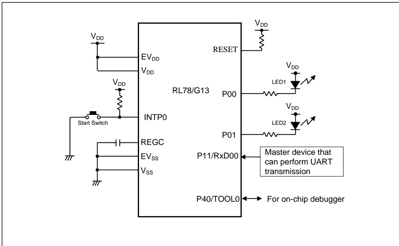
**Figure 4.1 Hardware Configuration**
