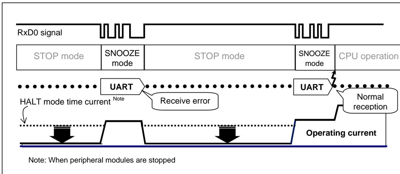
Figure 1.2 Outline of UART Receive Operation in SNOOZE Mode
