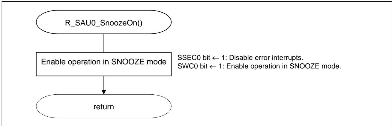
Figure 5.10 Enabling UART0 Operation in SNOOZE Mode
