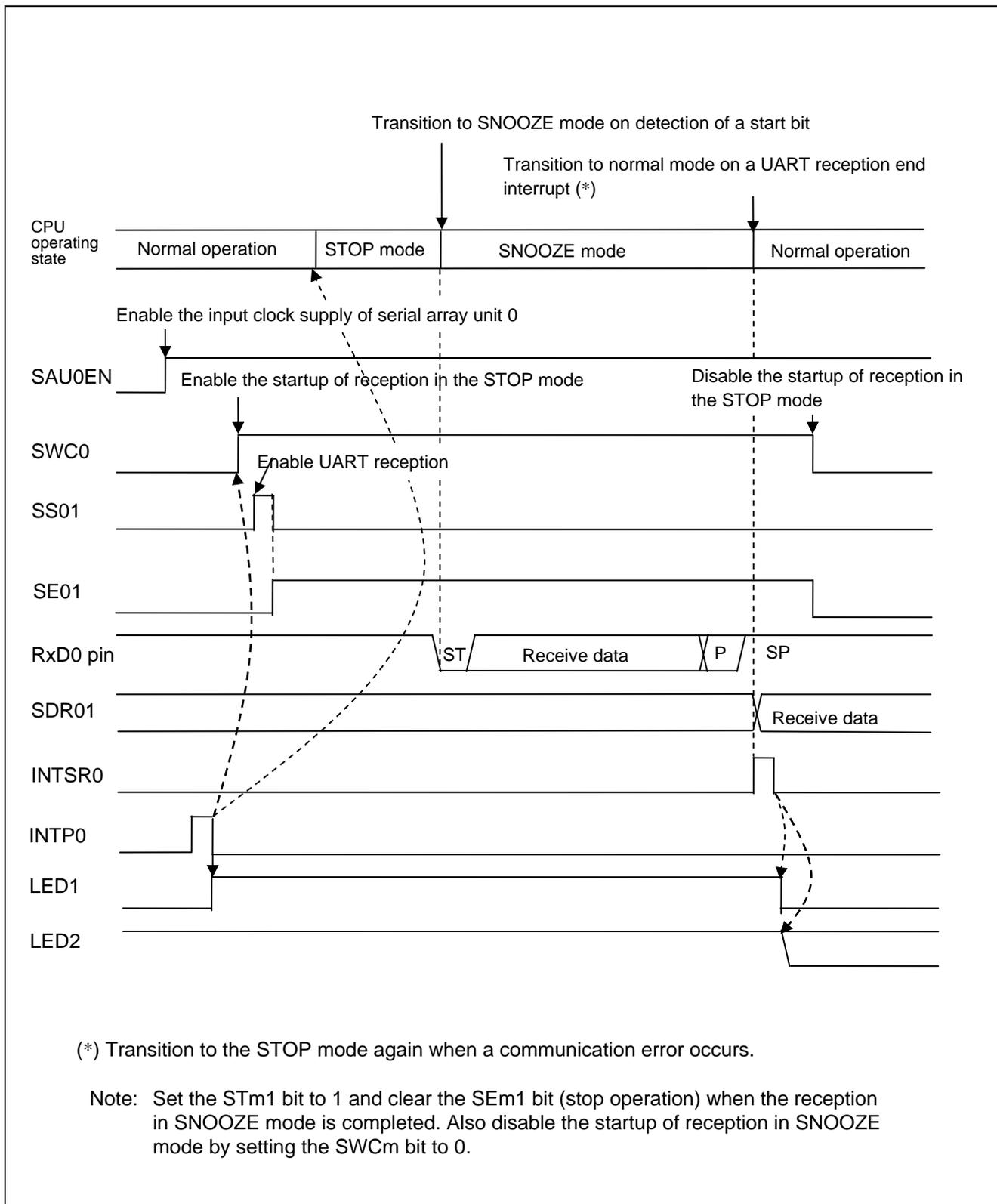
Figure 1.3 Timing Chart of SNOOZE Mode Operation
