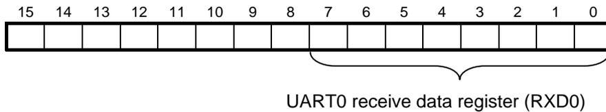
The receive data is written to the lower 8 bits of SDR01.
