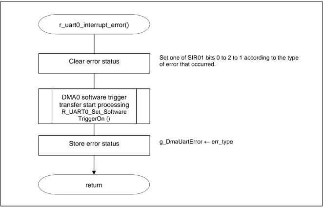
Figure 5.13 UART0 Reception Error Interrupt Processing
