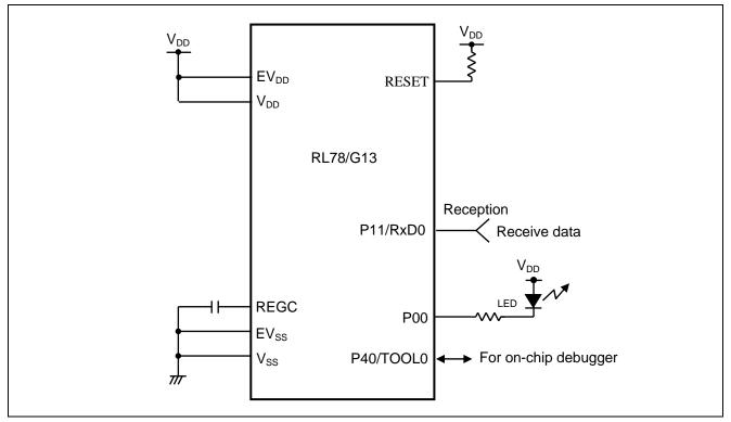
Figure 4.1 Hardware Configuration
