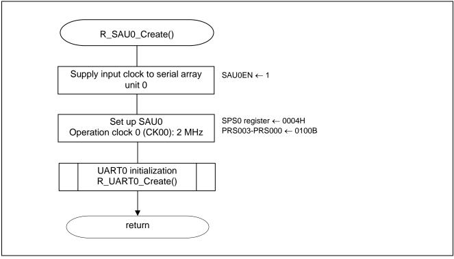
Figure 5.6 Serial Array Unit 0 Setup
