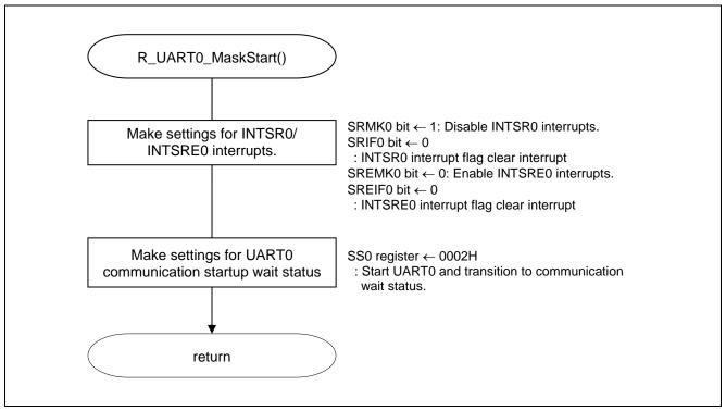
Figure 5.10 UART0 Communication Start Processing
