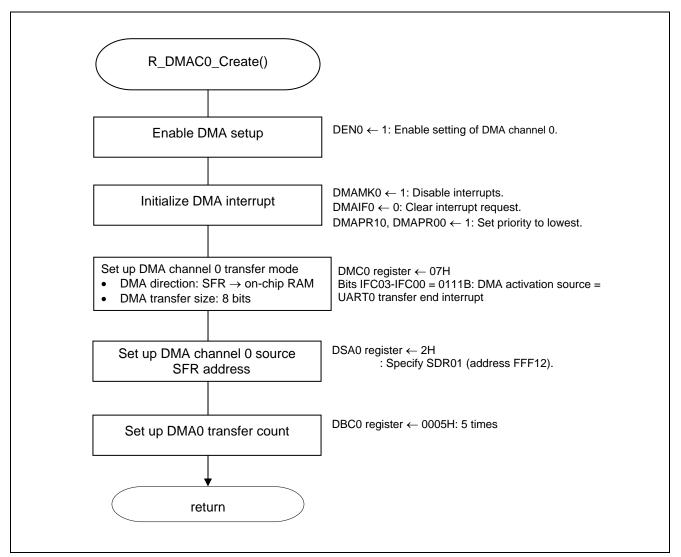
Figure 5.8 DMA Controller Initialization
