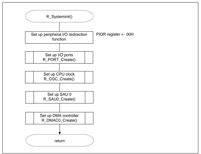
Figure 5.3 System Initialization Function
