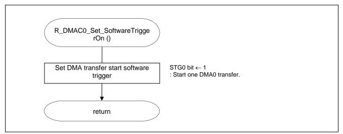
Figure 5.14 DMA0 Software Trigger Transfer Start Processing
