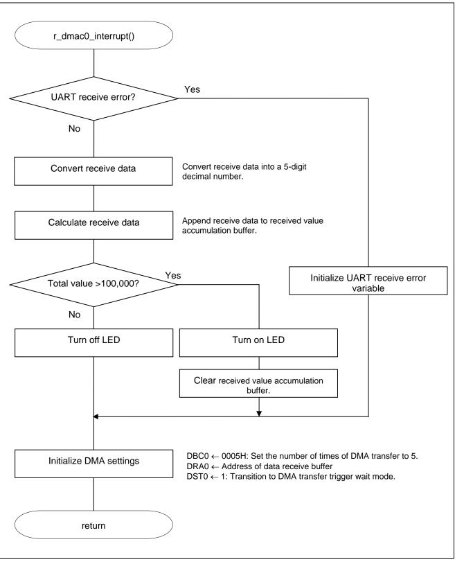
Figure 5.12 DMA0 Transfer End Interrupt Processing
