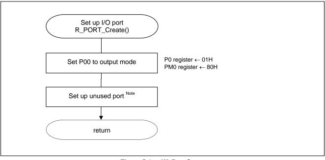
Figure 5.4 I/O Port Setup
