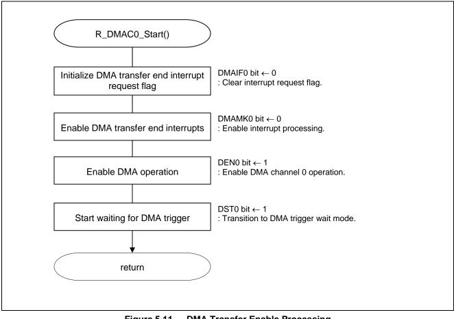
Figure 5.11 DMA Transfer Enable Processing
