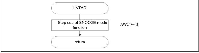
Figure 5.40 A/D Conversion Completion Interrupt Servicing
