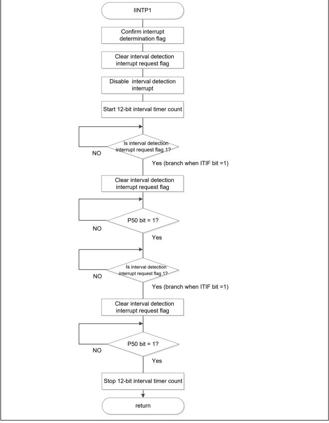
Figure 5.38 External Interrupt Servicing
