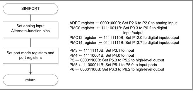
Figure 5.3 Input/Output Port Settings
