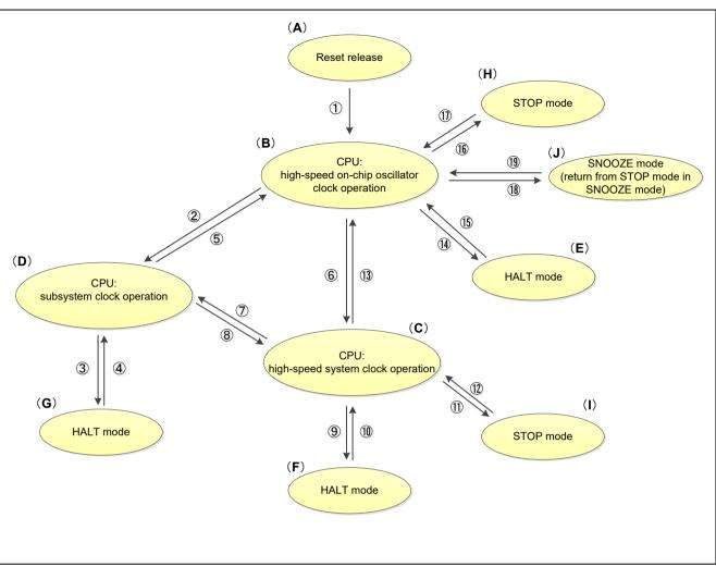
Figure 1.1 Operating Mode Status Transition Diagram
