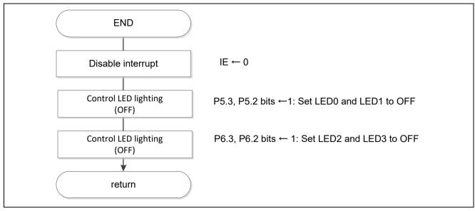
Figure 5.37 Status Transition End Processing
