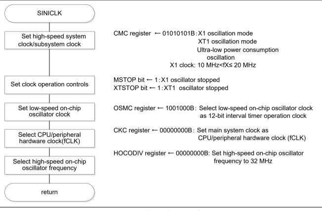
Figure 5.4 Clock Generator Setting
