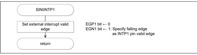
Figure 5.5 External Interrupt Setting
