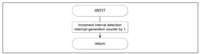
Figure 5.39 12-bit Interval Timer Interrupt Servicing
