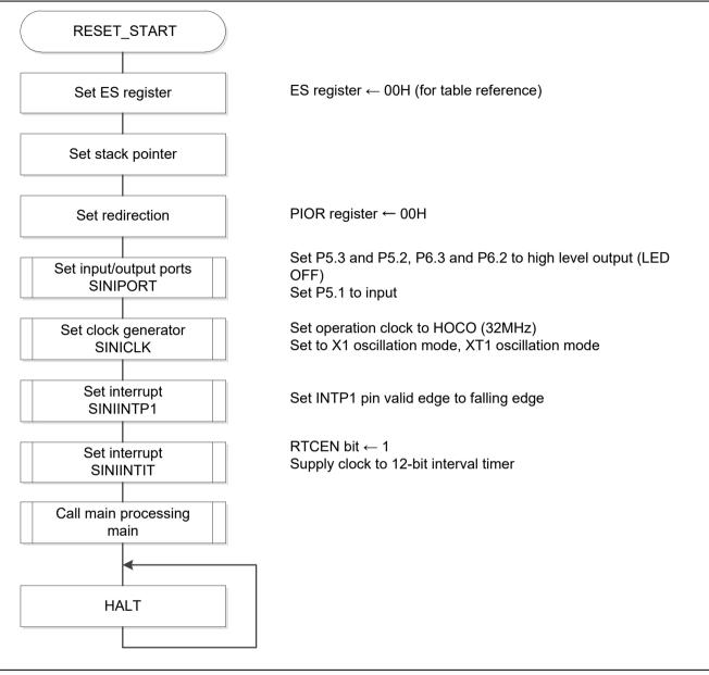
Figure 5.2 CPU Initialization Function
