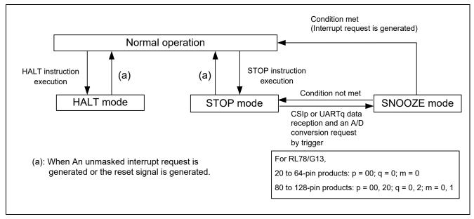
Figure 1.2 The state transitions of the RL78/G13 standby function
