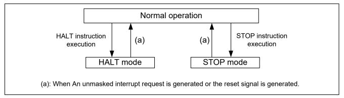
Figure 1.1 The state transitions of the 78K0/Kx2 standby function
