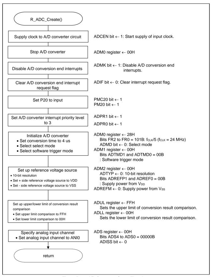
Figure 5.6 A/D Converter Setup Flowchart
