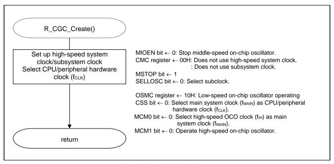
Figure 5.5 CPU Clock Setup
