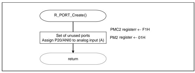
Figure 5.4 I/O Port Setup
