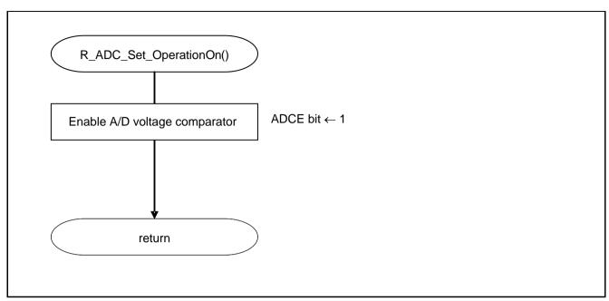
Figure 5.9 **Enabling the A/D Voltage Comparator**
