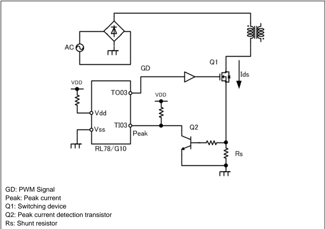
Figure 1-2 Peak Current Output Detection Using External Circuit
