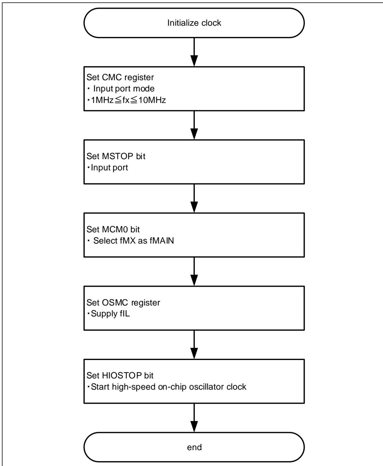
Figure 5-2 Clock Generation Circuit Initialization Flowchart
