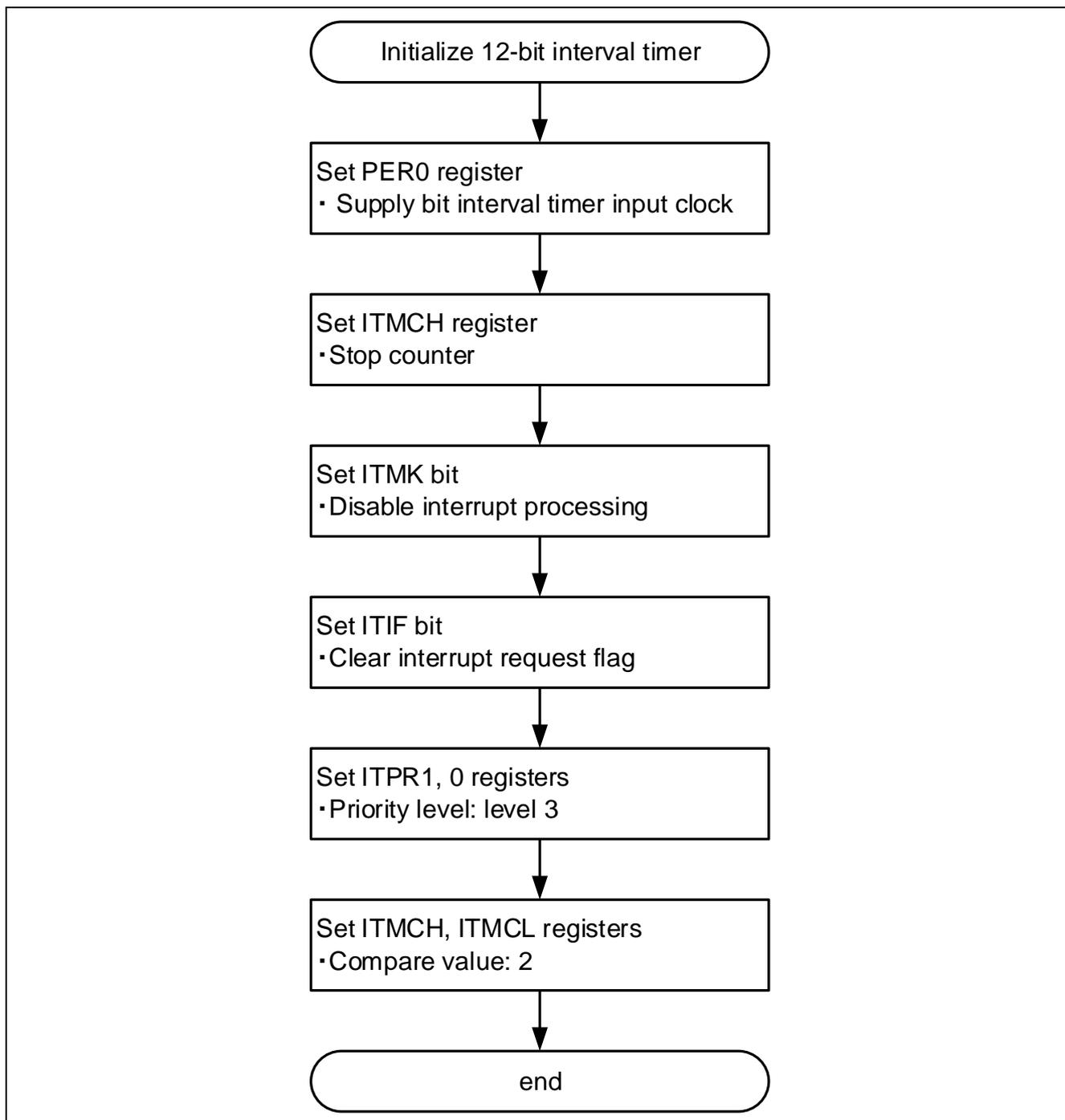
Figure 5-5 12-bit Interval Timer Initialization Flowchart
