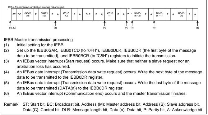
Figure 2-2 Master Transmission Processing (Timing Chart)
