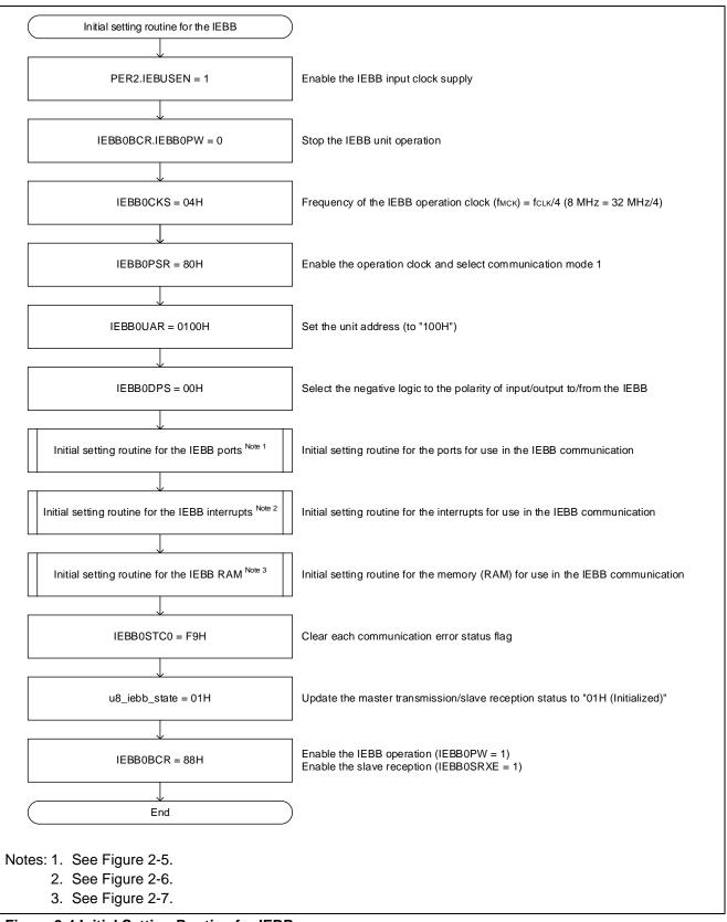
Figure 2-4 Initial Setting Routine for IEBB
