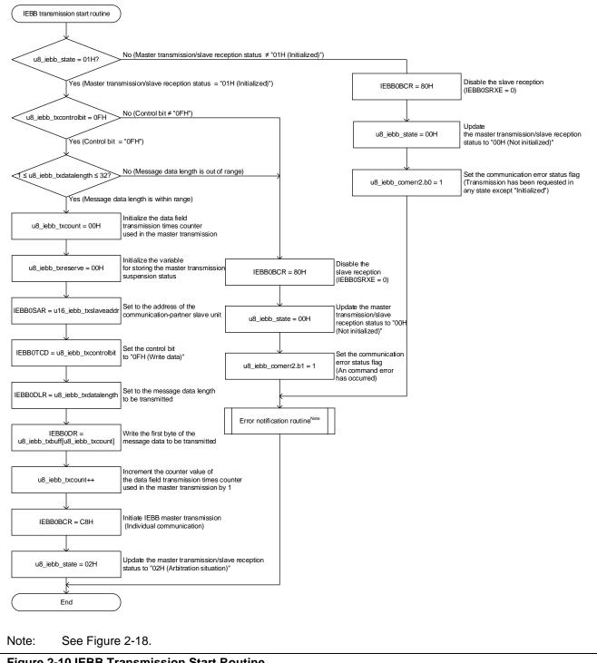
Figure 2-10 IEBB Transmission Start Routine
