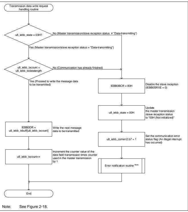
Figure 2-16 IEBus Transmission Data Write Request Handling Routine
