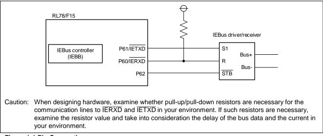
Figure 1-1 Pin Connections
