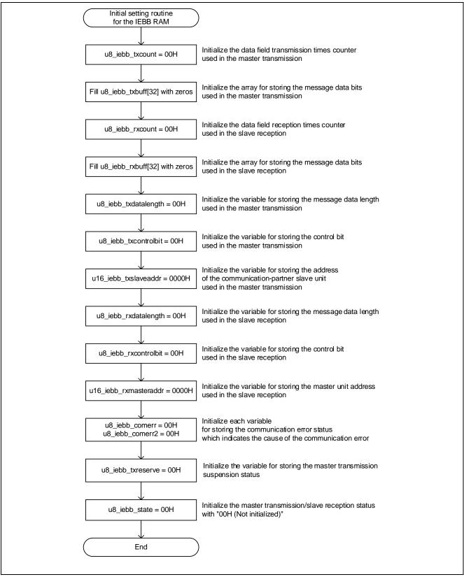
Figure 2-7 Initial Setting Routine for IEBB RAM
