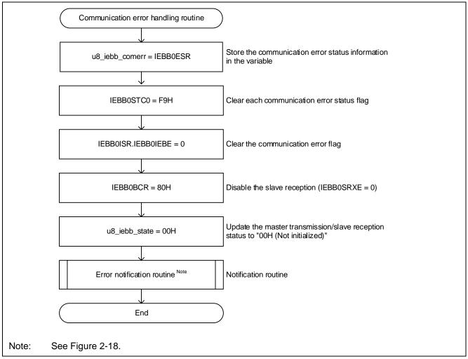
Figure 2-12 Communication Error Handling Routine
