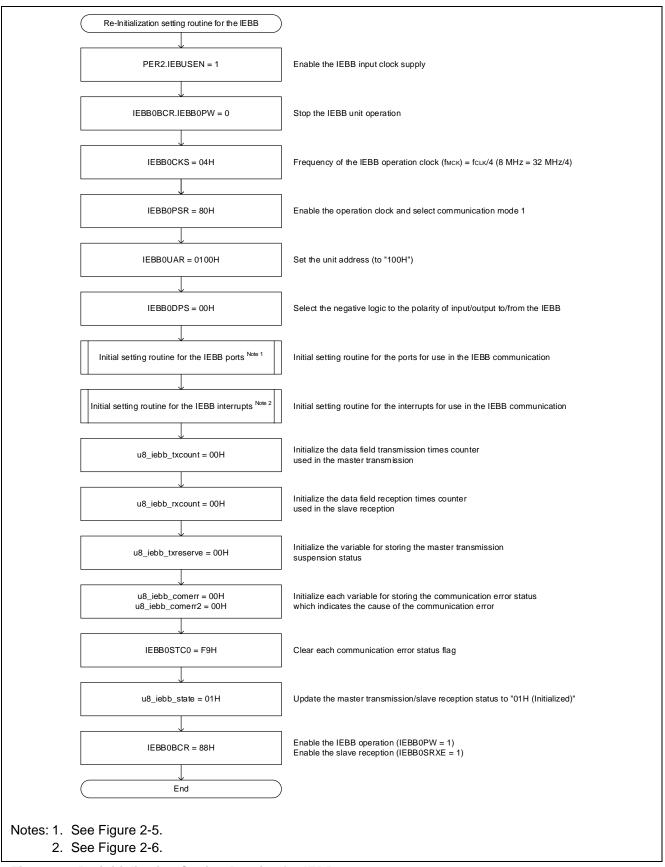
Figure 2-8 Re-initialization Setting Routine for IEBB
