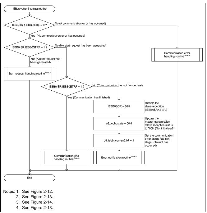
Figure 2-11 IEBus Vector Interrupt Routine
