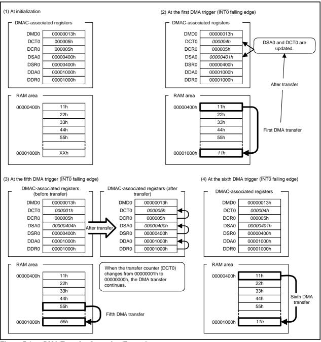
Figure 5.1 DMA Transfer Operation Example
