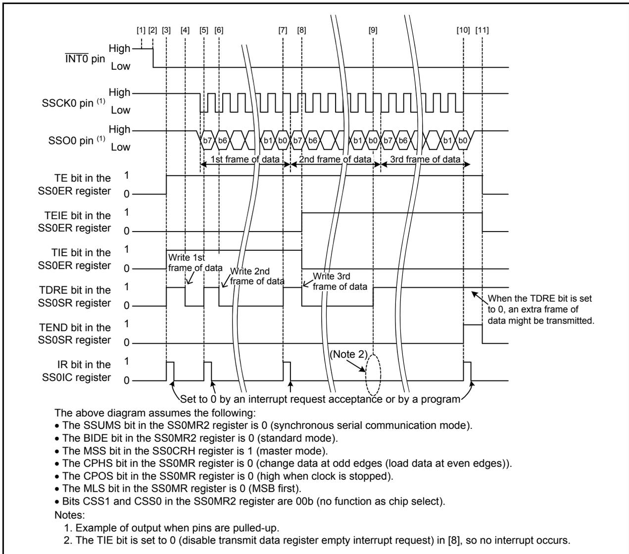
Figure 5.1 Master Transmission Timing Diagram
