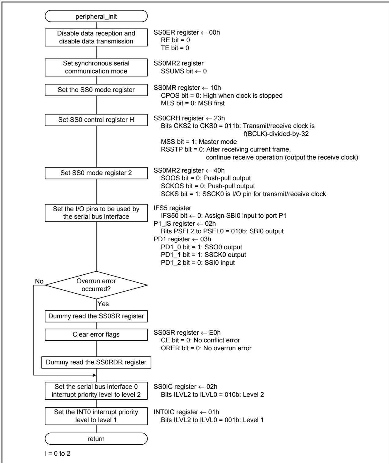
Figure 5.4 Initial Setting of the Peripheral Functions
