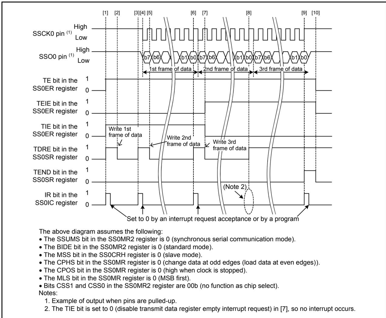
**Figure 7.2 Slave Transmission Timing Diagram**
