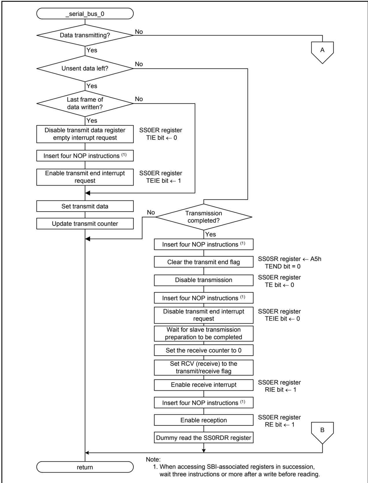
Figure 5.5 Serial Bus Interface 0 Interrupt Handling (1/2)
