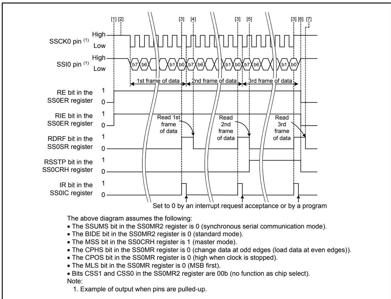
Figure 5.2 Master Reception Timing Diagram
