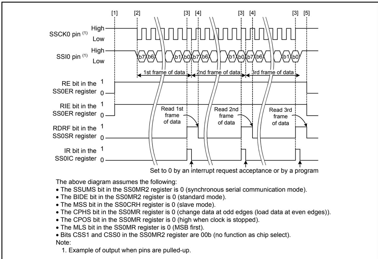
Figure 7.1 Slave Reception Timing Diagram
