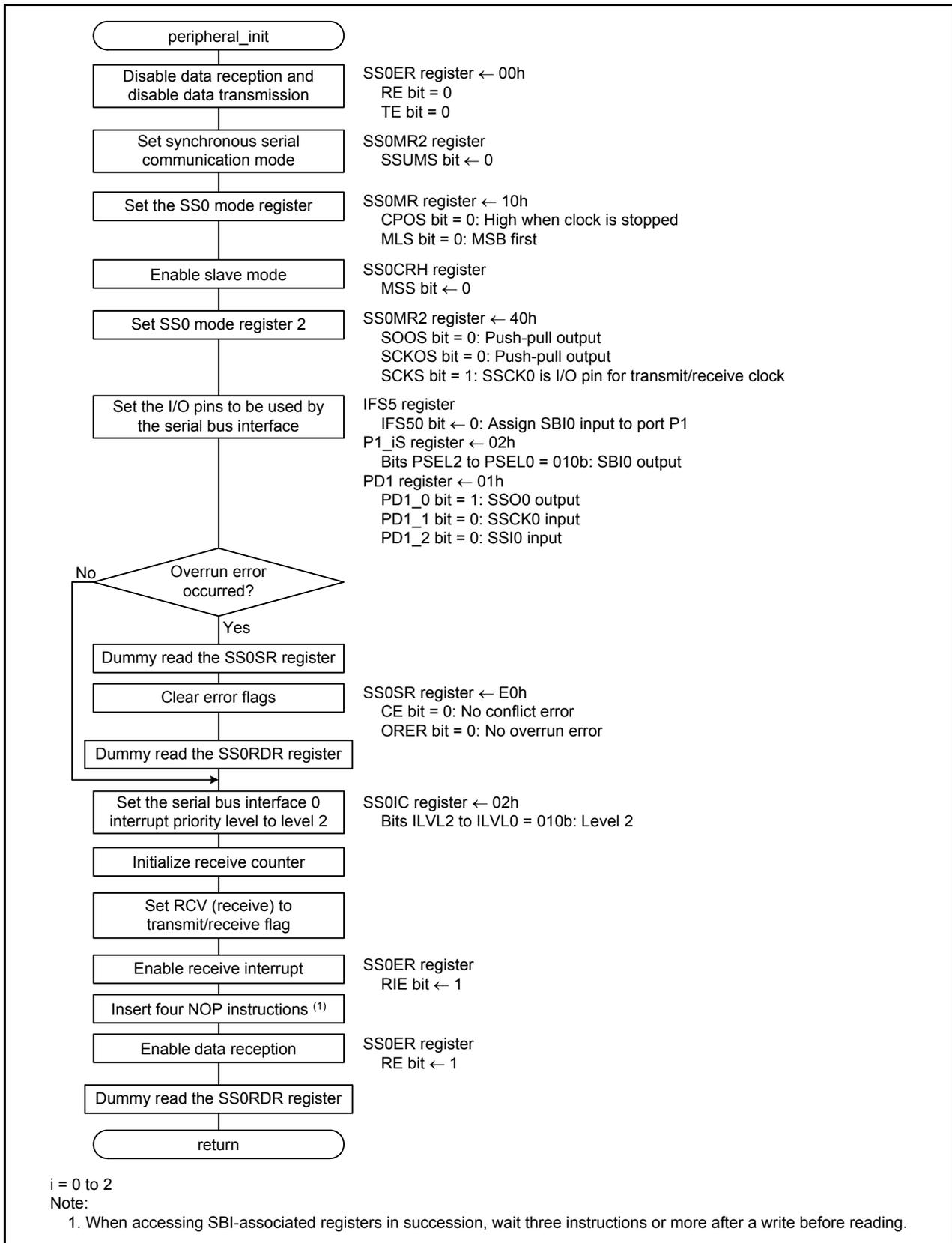
Figure 7.4 Initial Setting of the Peripheral Functions
