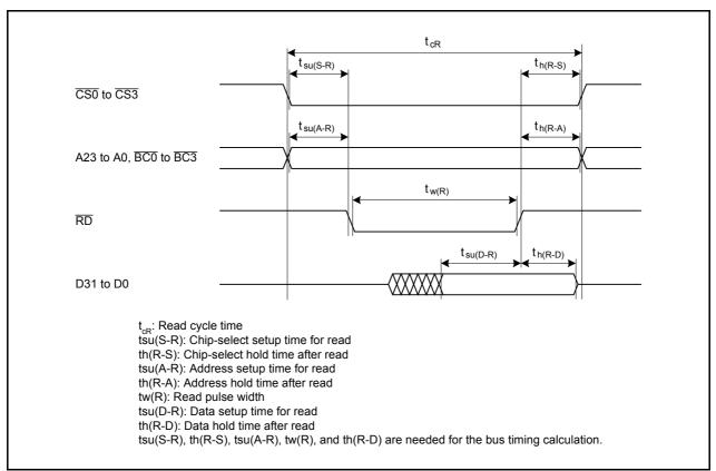
Figure 4.1 Read Cycle of the R32C/100 Series
