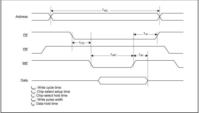
Figure 4.5 Example of External Device Bus Timing When Writing
