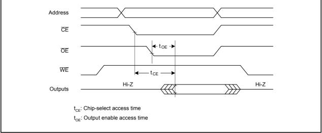
Figure 4.2 Example of External Device Bus Timing When Reading
