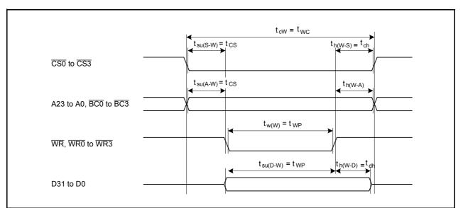
Figure 4.6 Write Bus Timing Comparison between the R32C/100 Series and the External Device
