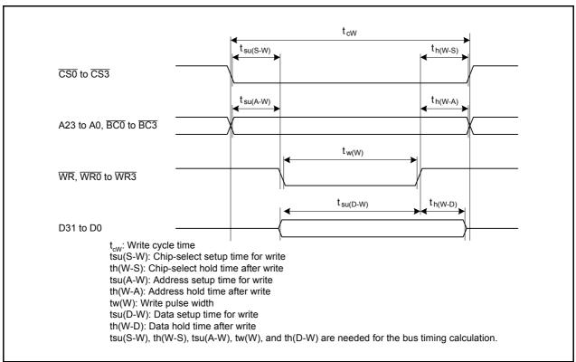
Figure 4.4 R32C/100 Series Write Cycle
