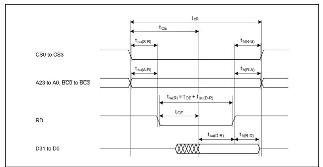
Figure 4.3 Read Bus Timing Comparison between the R32C/100 Series and an External Device
