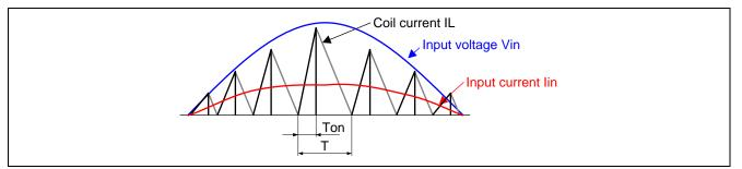
Figure 7.2 Input Current & Inductor Current
