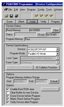
**Figure 3 Device Configuration Window**
