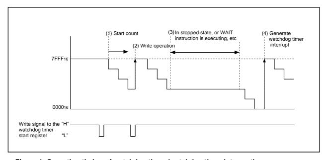
Figure 1. Operation timing of watchdog timer (watchdog timer interrupt)
