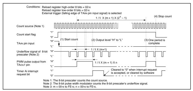
Figure 1. Operation timing of pulse width modulation mode, with 8-bit PWM mode
