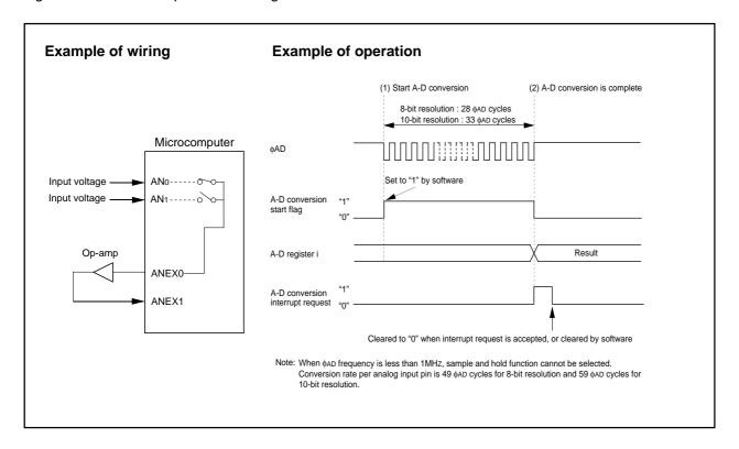
Figure 1. Operation timing of one-shot mode, with external op-amp connection mode selected
