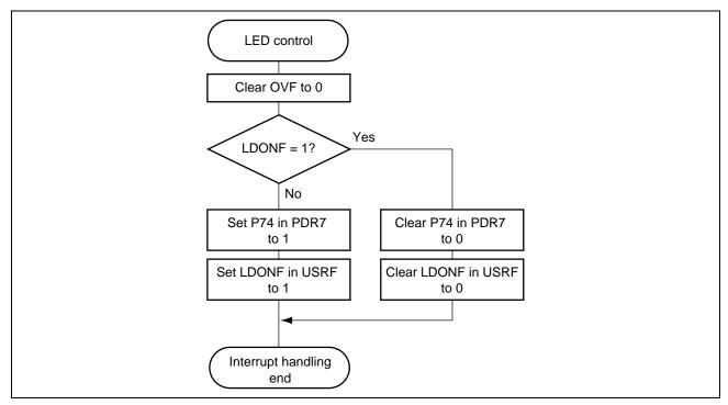
Figure 4 Flowchart for Timer V Interrupt Handling Routine
