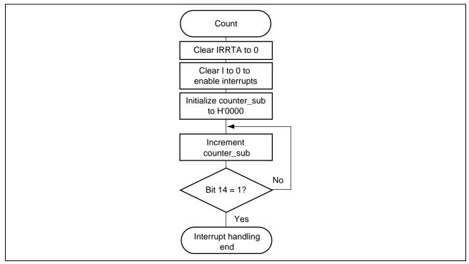
Figure 3 Flowchart for Timer A Interrupt Handling Routine
