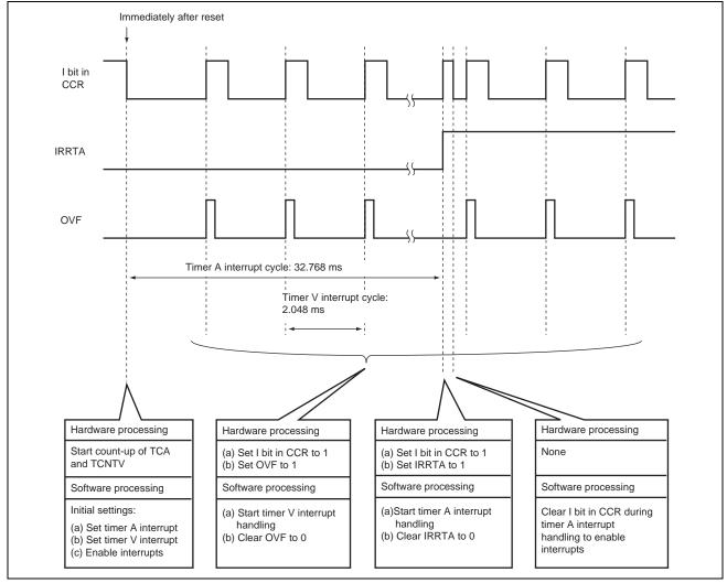
Figure 1 Operation Principle: Multi-Interrupt Operation with Internal Interrupts
