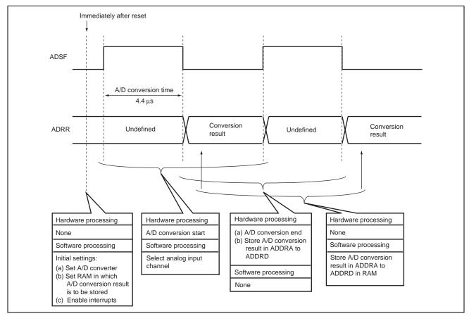
Figure 3 Operation Principle: Voltage Measurement by 4-Channel A/D Conversion
