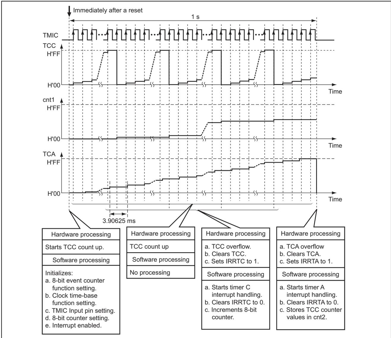
Figure 2 Operation Principle of Frequency Measurement by Timer C 8-bit Event Counter Function
