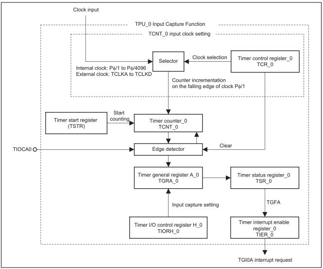
Figure 2 Block Diagram of TPU Channel 0 (TPU\_0)
