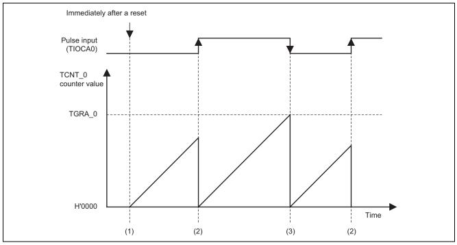
Figure 3 Operation Principles of High and Low Pulse Width Measurement
