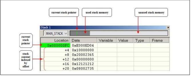
Figure 8 Graphical representation of stack usage
