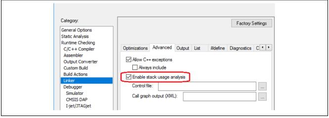
Figure 1 Enable stack usage analysis
