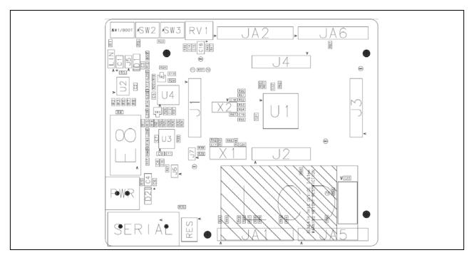
Figure 5 Connectors placement of Renesas Starter Kit CPU Board for R8C/2D
