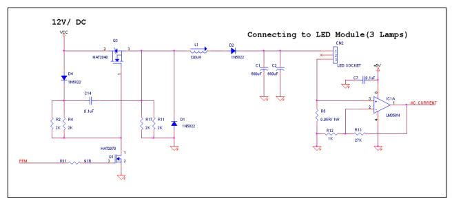
**Figure 8 PFM Control Circuit**
