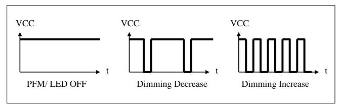
Figure 4 PFM Dimming Signals
