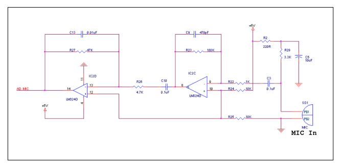
Figure 9 MIC in Sensing Circuit
