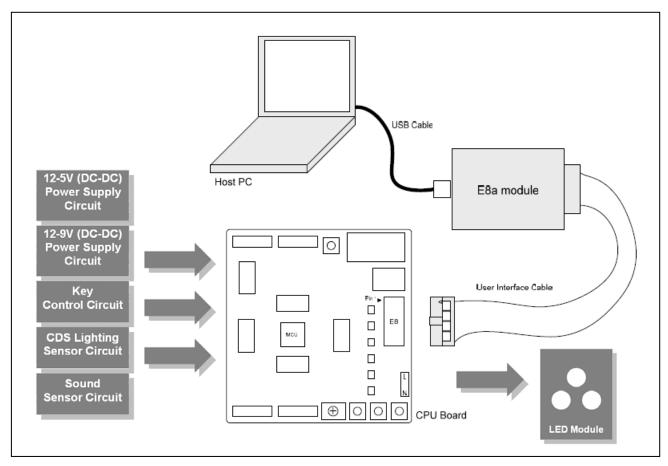
Figure 2 Implement LED table lighting application on RSK R8C/2D
