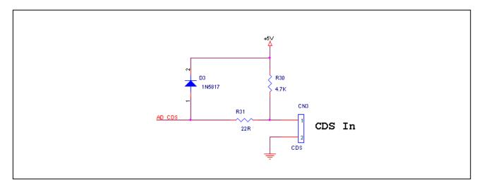
**Figure 10 CDS Sensing Circuit**
