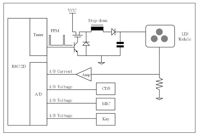
Figure 3 R8C/2D Timer RF out PFM Circuit
