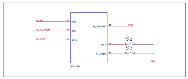
Figure 6 R8C/2D Control Schematics
