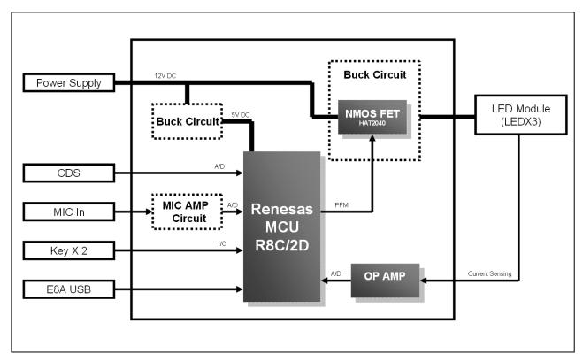
Figure 1 the configuration of the system
