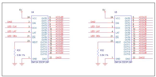
Figure 8 Serial to Parallel Shifter of Column Data (1)
