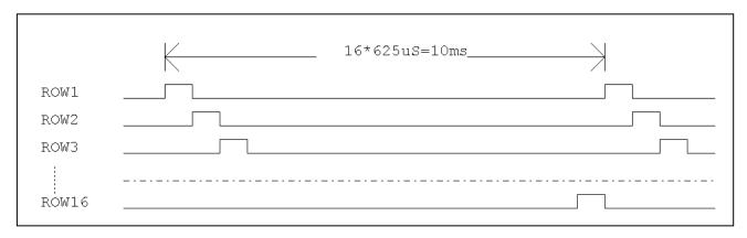
Figure 5 Row Scan Line Timing
