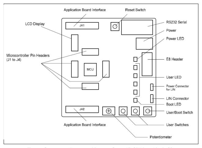
Figure 6 Connectors placement of Renesas Starter Kit CPU Board for R8C/27
