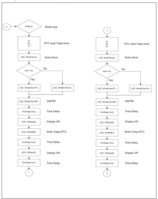
Figure 16 Program flow chart of while(1) loop routine
