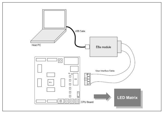
Figure 3 Implement LED digital clock application on RSK R8C/27
