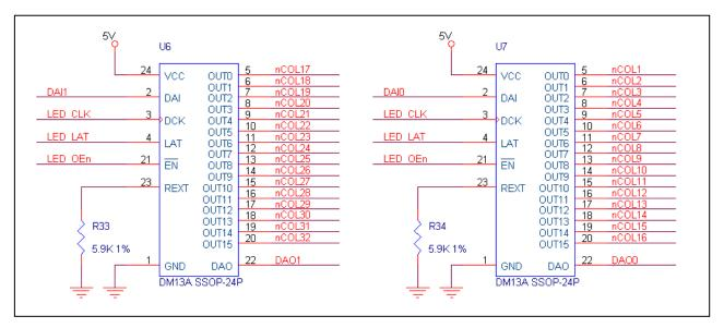
Figure 9 Serial to Parallel Shifter of Column Data (2)
