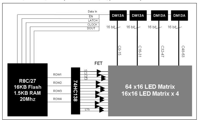
Figure 1 The configuration of the system
