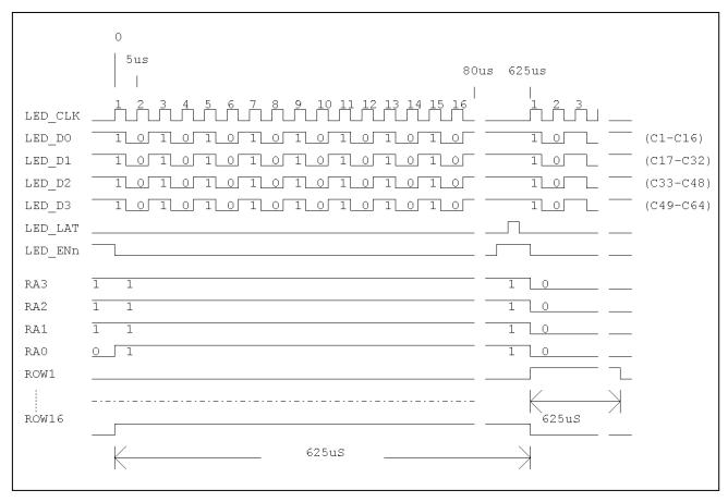
Figure 4 Column Data Shifter Timing
