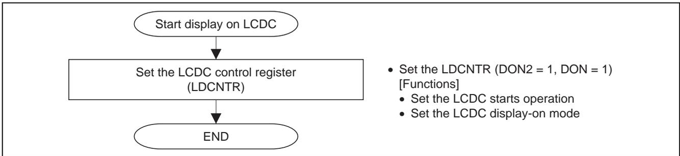
**Figure 13 Setting Examples of the Start of LCDC Display**
