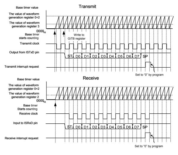
Figure 18 Clock Synchronous Serial I/O (UART) Output Timing Diagram
