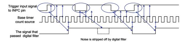
Figure 5 Digital Filter Operation Timing Diagram
