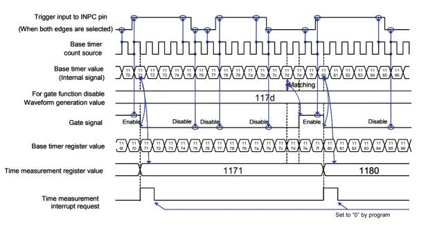
Figure 6 Gate Function Operation Timing Diagram
