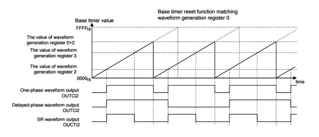
Figure 10 Base Timer Reset Function Operation Diagram
