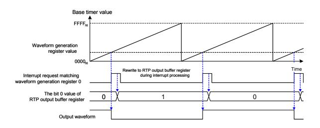
Figure 14 Real-Time Port Output Timing Diagram
