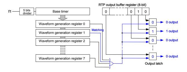
Figure 15 Parallel Real-Time Port Output Schematic Drawing
