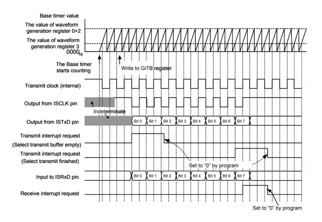
Figure 17 Clock Synchronous Serial I/O Output Timing Diagram
