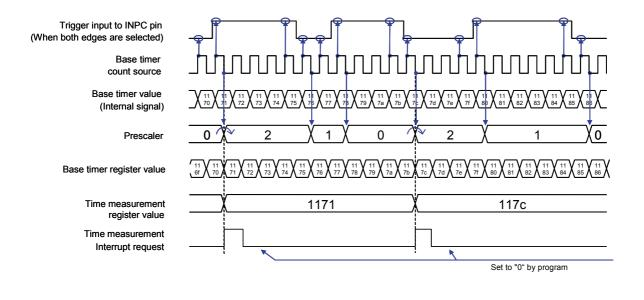
Figure 7 Prescaler Operation Timing Diagram
