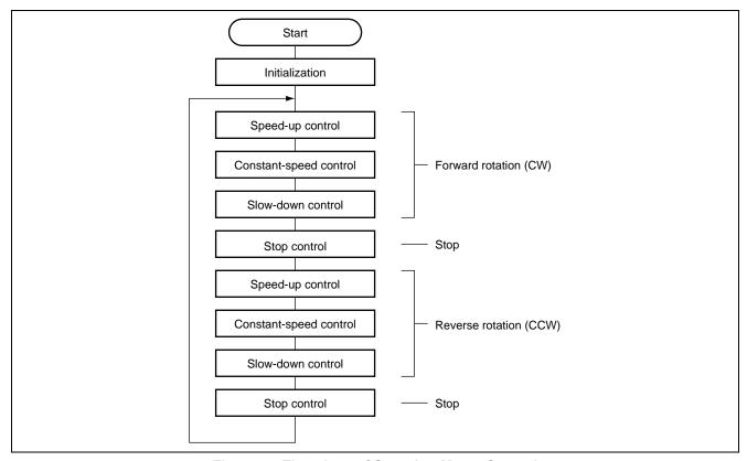
Figure 7 Flowchart of Stepping Motor Control
