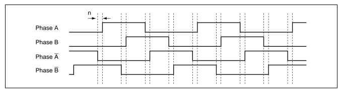
Figure 5 Example of Output with Non-Overlap Time
