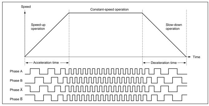
Figure 6 Speed-Up and Slow-Down Operation
