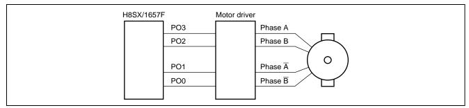
Figure 1 Connections for Two-Phase Stepping Motor Control
