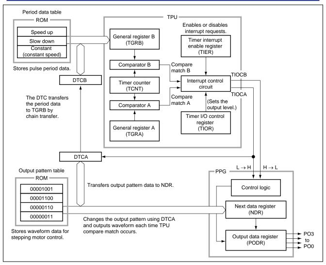
Figure 2 H8SX/1657F's Functions Used in This Application
