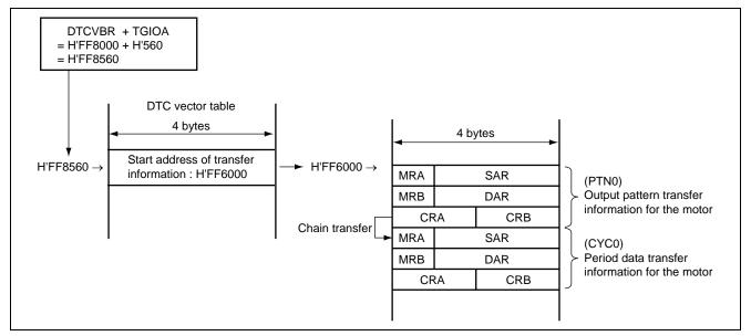
Figure 3 Example of DTC Vector Table and Data Arrangement in Memory
