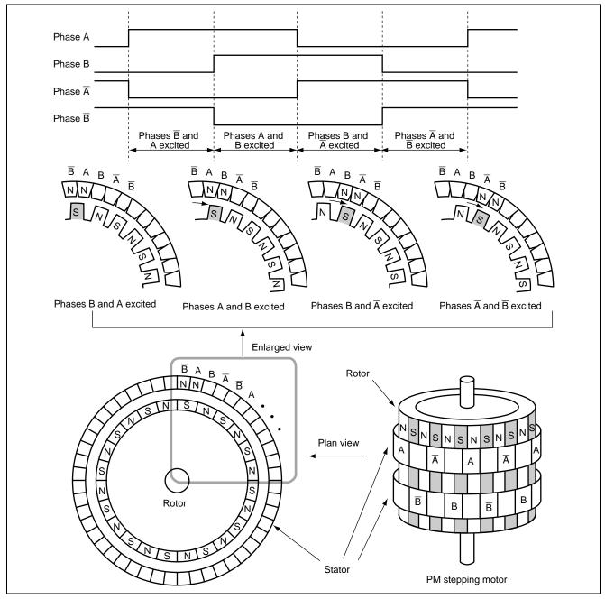
Figure 4 Example of Stepping Motor Operation
