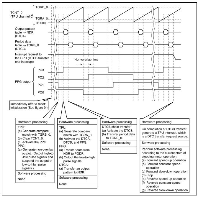
Figure 8 Timing of Stepping Motor Operation
