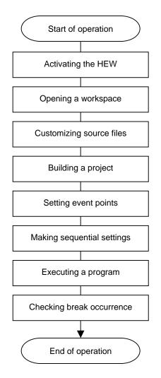
Figure 4.1 Procedures for Sample Program Execution
