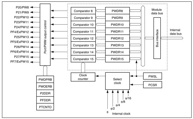
Figure 2 Block Diagram of 8-bit PWM Module
