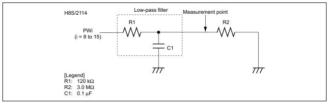
Figure 1 Example Circuit for Use as a D/A Converter
