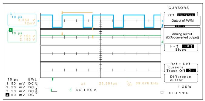
Figure 4 D/A-Converted Waveform Generated by Using the 8-bit PWM Function (for Reference)
