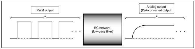
Figure 3 Operation of a D/A Converter Driven by the 8-bit PWM Function
