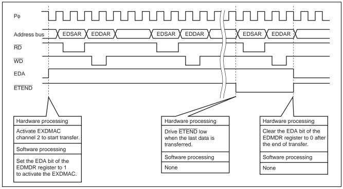
Figure 3 Example of Normal Transfer Operation
