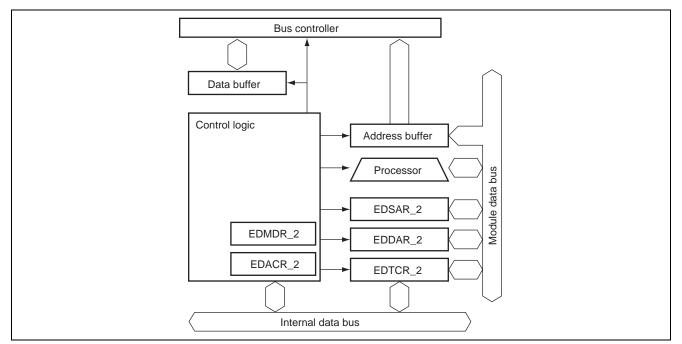
Figure 2 Block Diagram of EXDMAC
