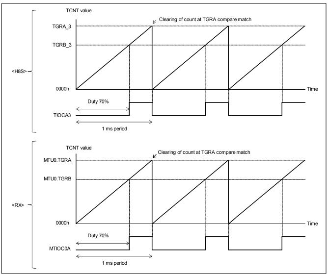
Figure 3.3 Example of PWM Mode 1 Operation on H8S/2378 Group and RX231 Group
